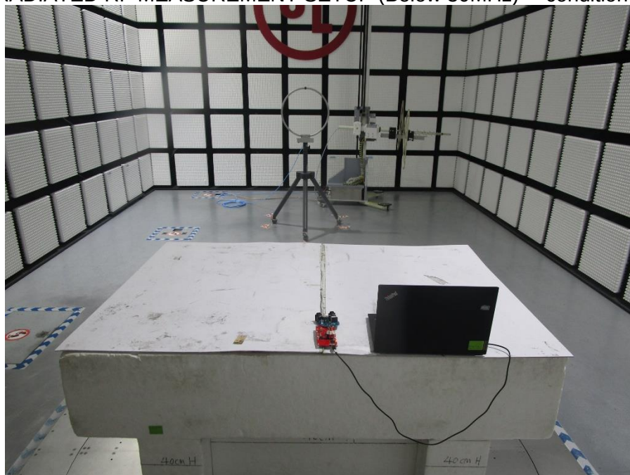
RADIATED RF MEASUREMENT SETUP (Below 30MHz) ---condition 3
