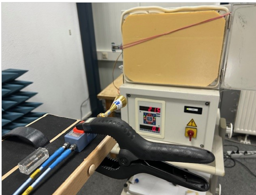
Photograph 10: EUT test setup in the RC8G Lab_climate cabinet
