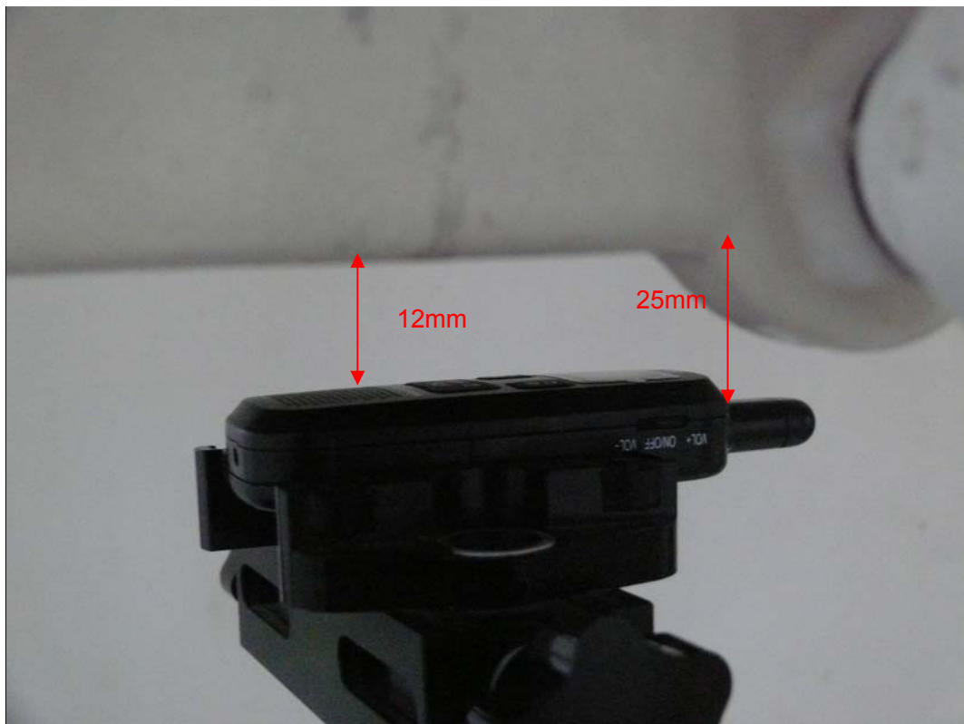
Picture 4: Face-held, The EUT display towards phantom, the distance from EUT Antenna to the bottom of the Phantom is 25mm
