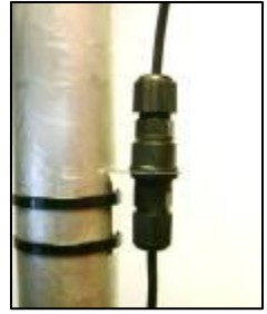
Figure 27 - RJ45 Seal Kit installation
