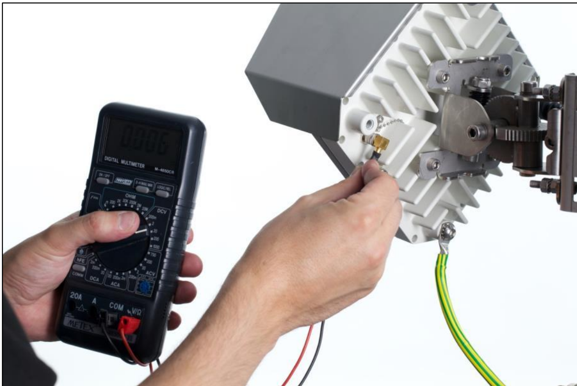
Figure 34 - Connection of a voltmeter for fine alignment on Liberator-V1000
