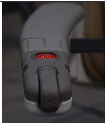
Photo 4: Front view of UI-Joystick module mounted in armrest, joystick folded down, unusable position (park/boarding position)
