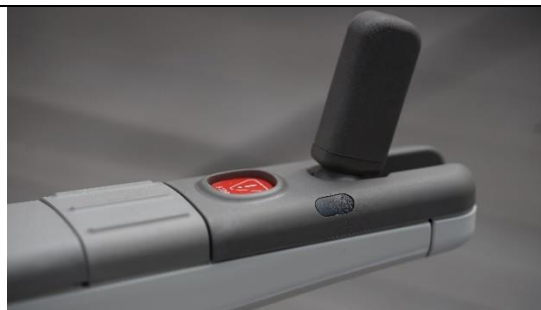
Photo 2: UI-Joystick module mounted in left armrest, joystick in upright position
