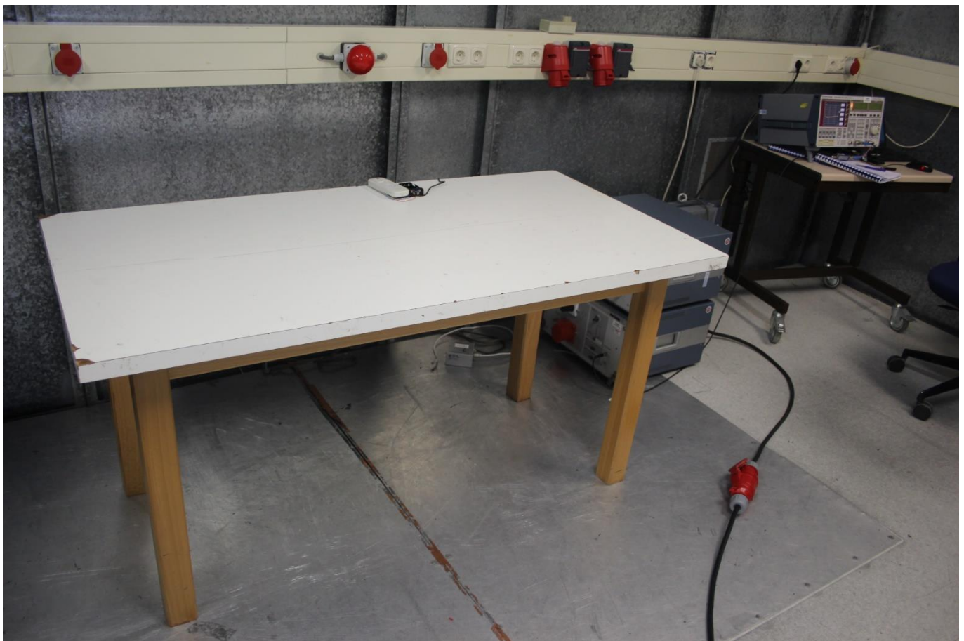
Figure 4. AC Power Line conducted emissions setup
