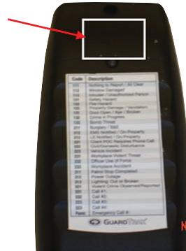
**3** The GT2 has now read the RFID tag. After reading the RFID tag, the LCD will show “RFID OK”, indicating a positive read, and the GT2 immediately uploads the tag information to the GuardTrax web site (assuming you have GSM connection).
