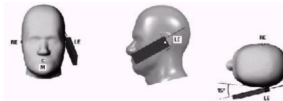
Figure 12.6 Front, Side and Top View of Ear/15 Tilt Position
