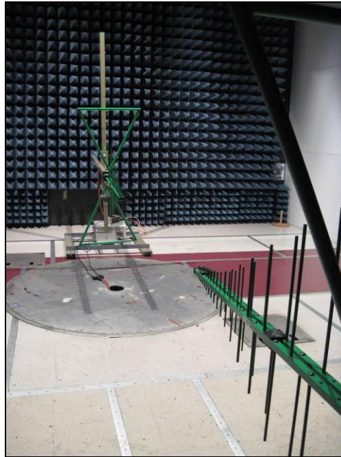
Photograph 1. EIRP, Test Setup, 850 MHz
