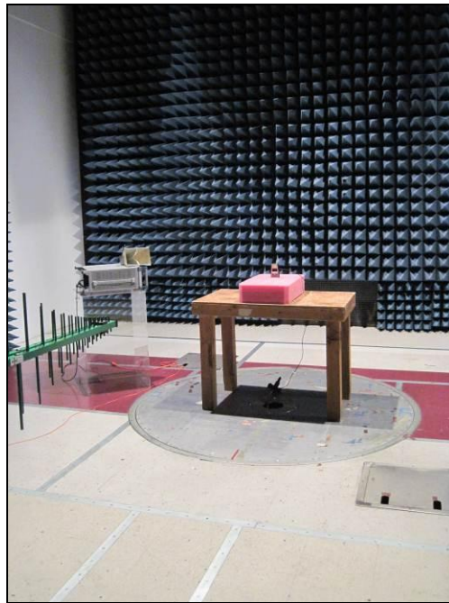
Photograph 3. Radiated Emissions, Test Setup, Below 1 GHz
