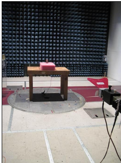
Photograph 4. Radiated Emissions, Test Setup, Above 1 GHz
