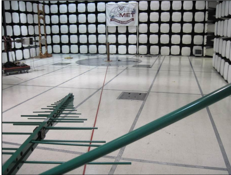
Photograph 3. Radiated Emission, Test Setup, 30 MHz – 1 GHz
