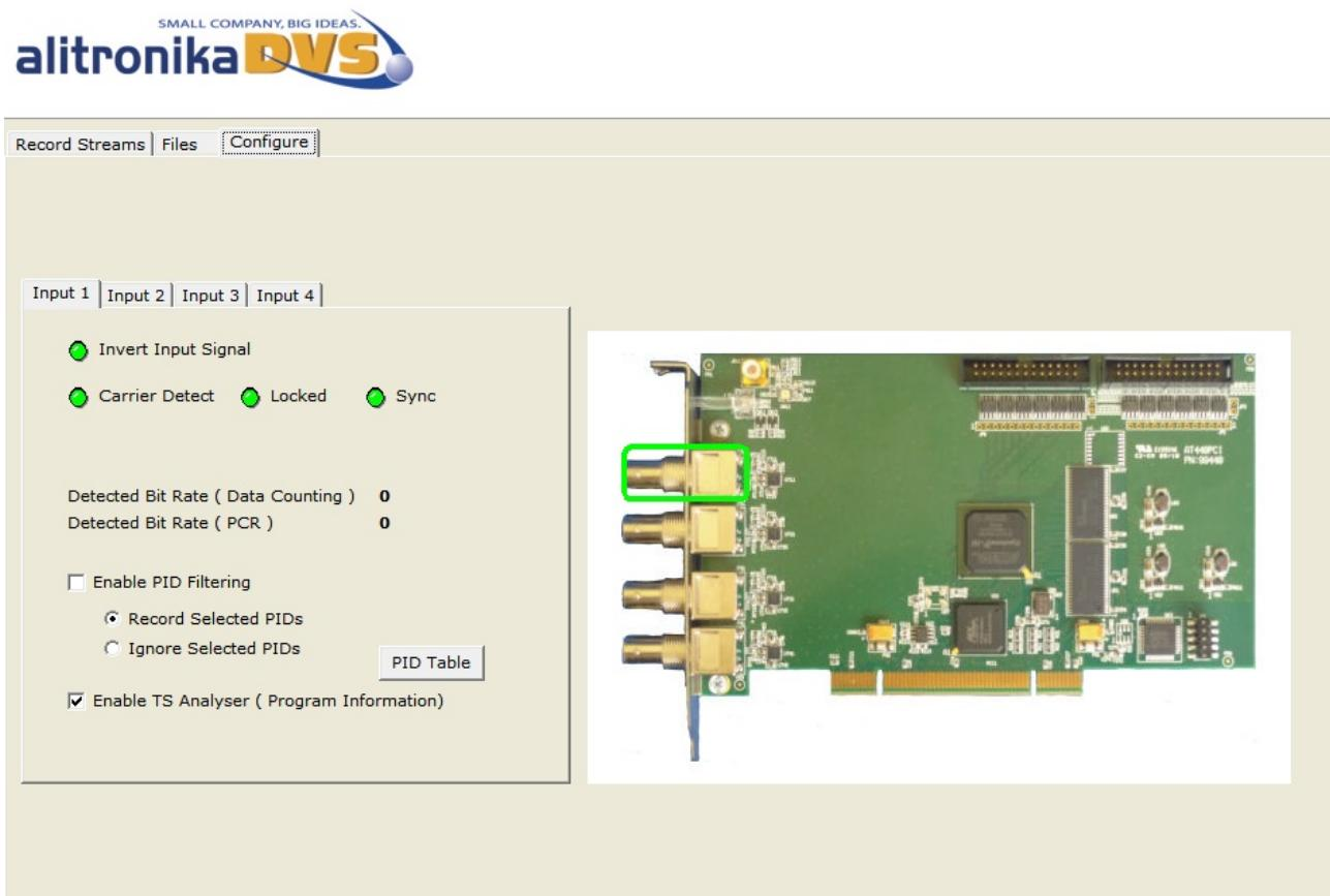
The enable TS Analyser (Program Information) allow the analysis of the transport stream for program information to be turned on and off on a channel by channel basis.
