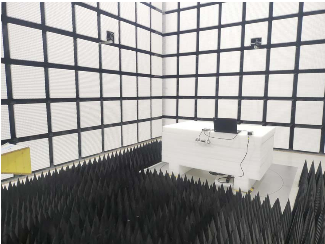
Radiated Emission Above 1GHz Rear View-Chip Antenna
