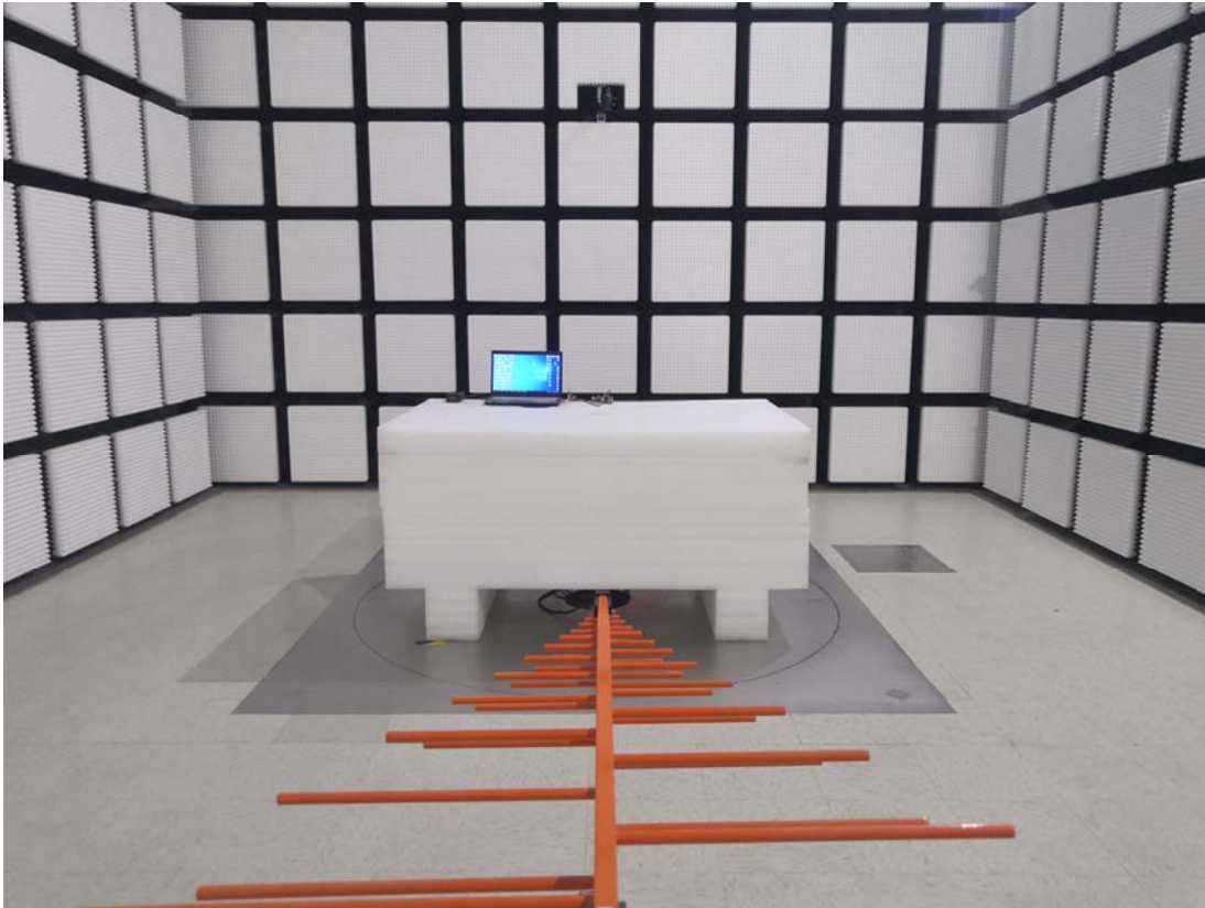
Radiated Emission Below 1GHz Rear View-Chip Antenna
