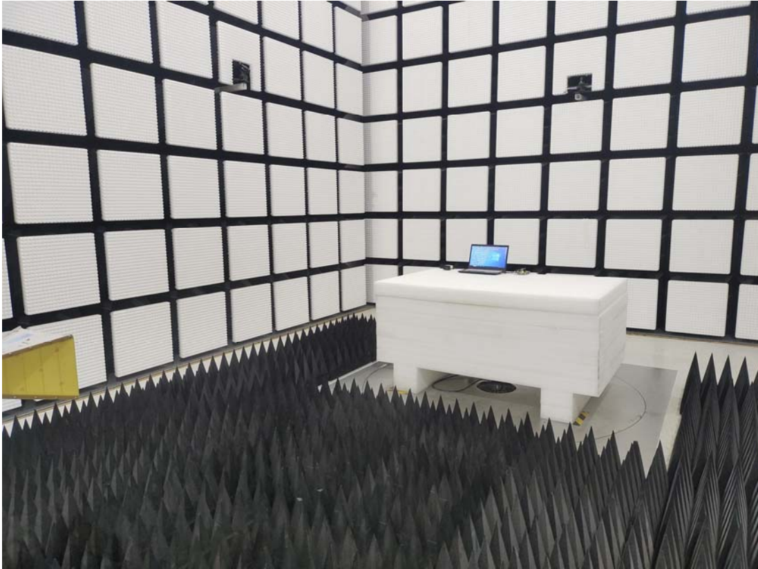
Radiated Emission Above 1GHz Rear View-Chip Antenna
