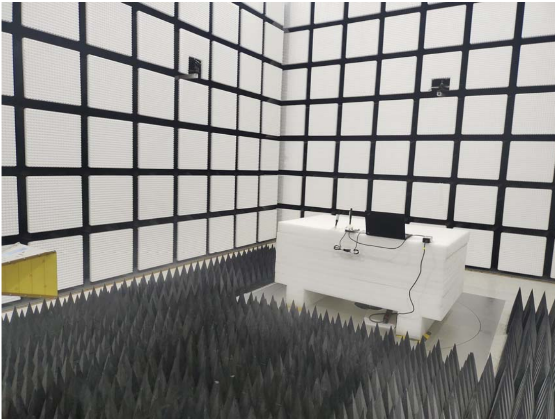
Radiated Emission Above 1GHz Rear View-Whip Antenna
