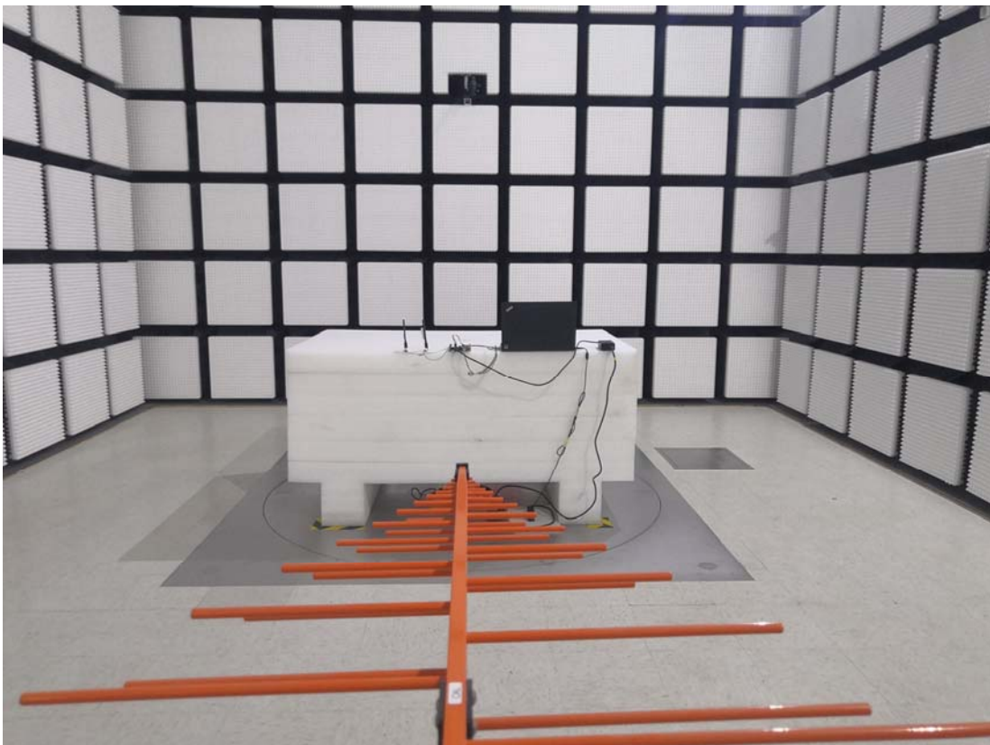
Radiated Emission Below 1GHz Rear View-Whip Antenna
