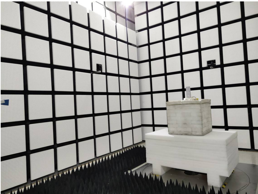
Radiated Emission 18-26.5GHz View POE
