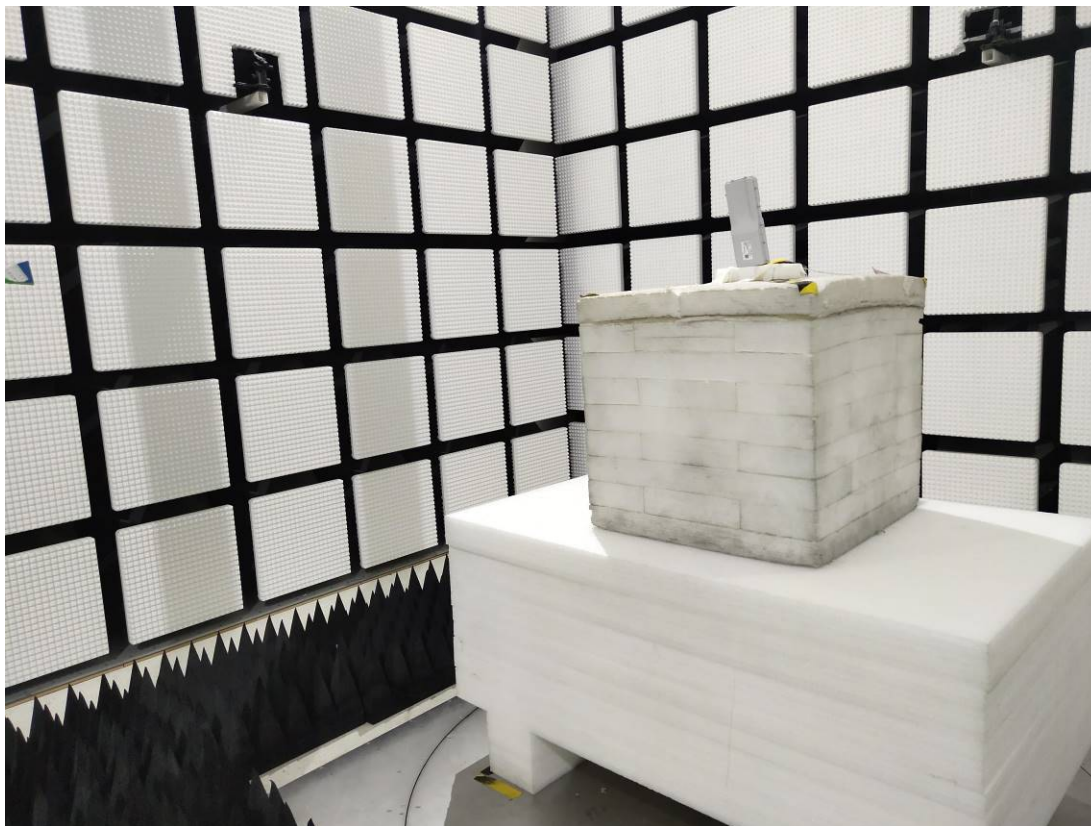
Radiated Emission 40-60GHz View POE
