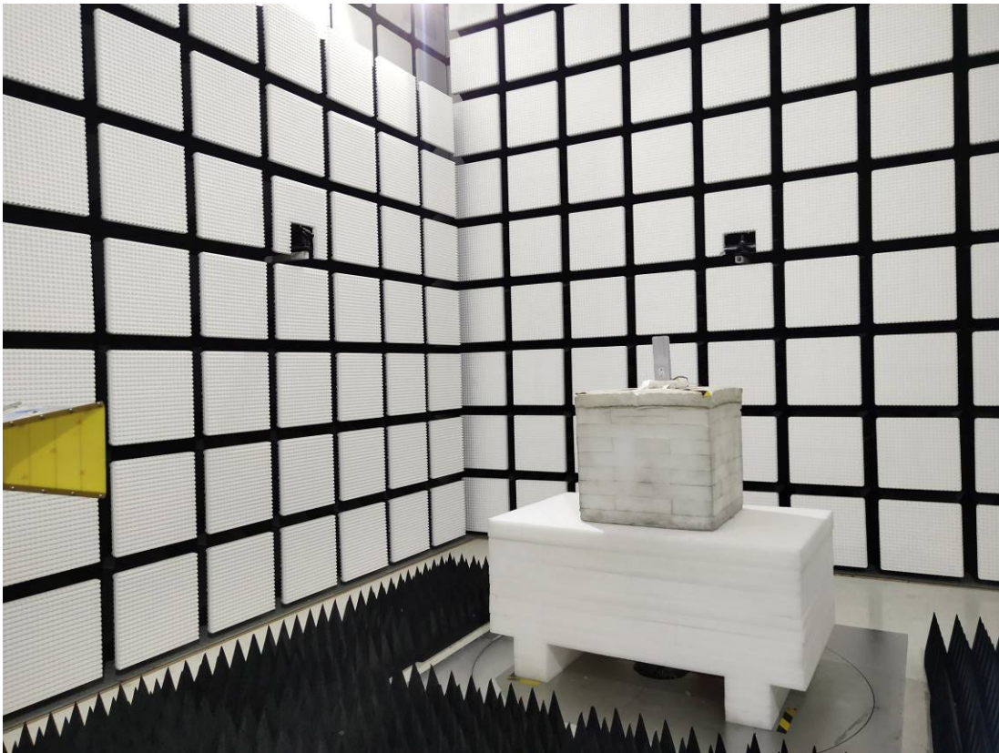
Radiated Emission 18-26.5GHz View POE
