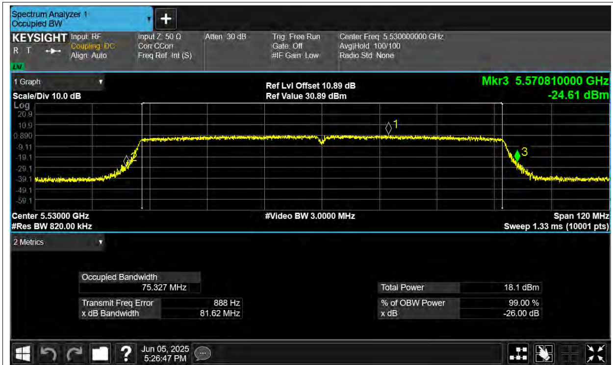
-26dB Bandwidth NVNT ac80 5530MHz Ant2
