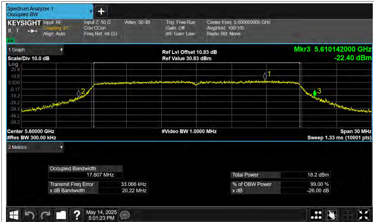
-26dB Bandwidth NVNT n20 5600MHz Ant4
