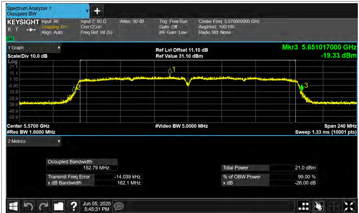
-26dB Bandwidth NVNT ac160 5570MHz Ant4
