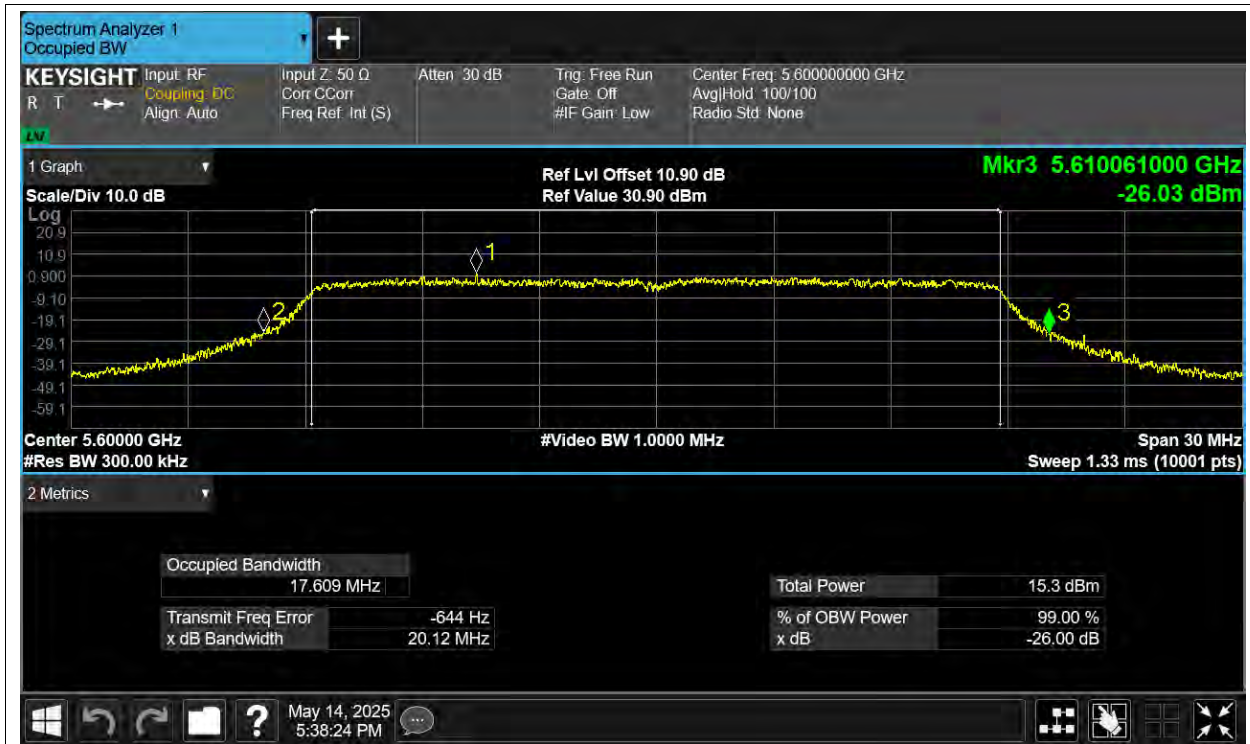
-26dB Bandwidth NVNT ac20 5600MHz Ant2
