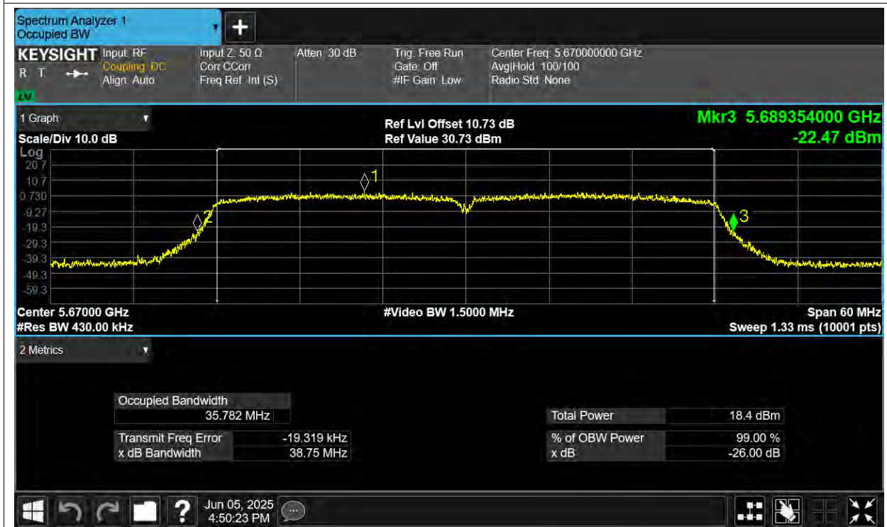
-26dB Bandwidth NVNT n40 5670MHz Ant3
