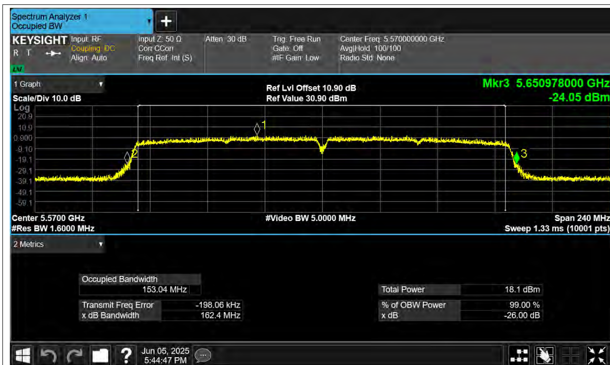
-26dB Bandwidth NVNT ac160 5570MHz Ant2
