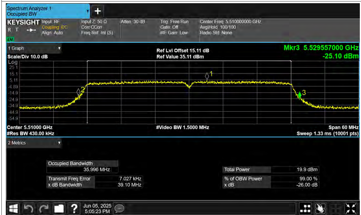
-26dB Bandwidth NVNT ac40 5590MHz Ant1
