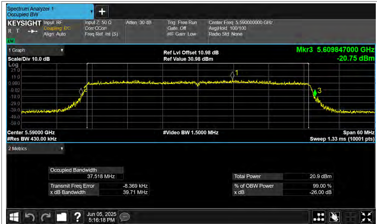
-26dB Bandwidth NVNT ax40 5590MHz Ant4
