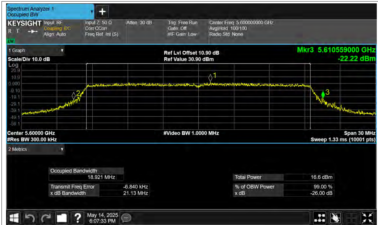
-26dB Bandwidth NVNT ax20 5600MHz Ant2
