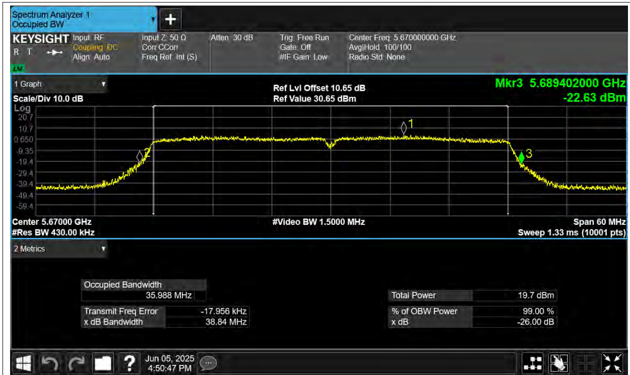
-26dB Bandwidth NVNT n40 5670MHz Ant4
