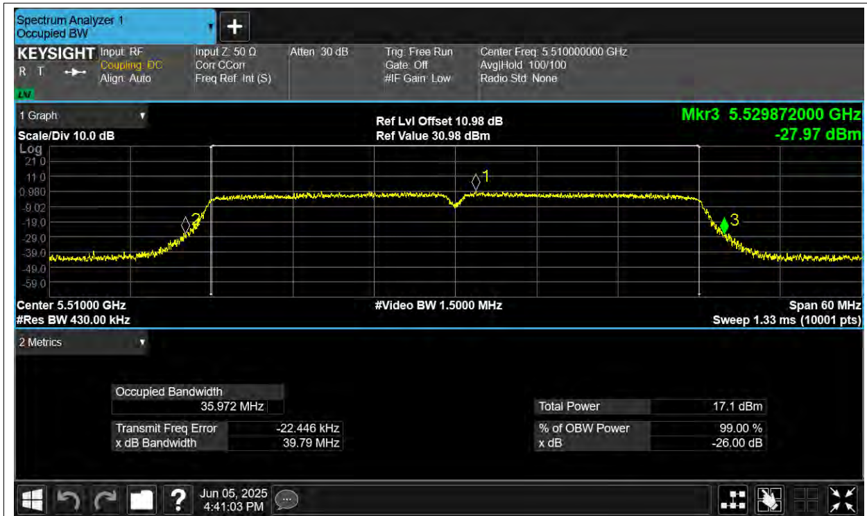
-26dB Bandwidth NVNT n40 5510MHz Ant2
