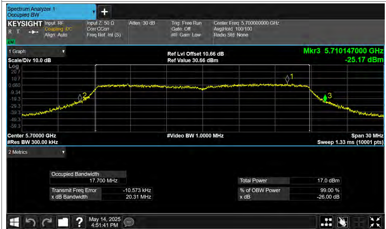
-26dB Bandwidth NVNT n20 5700MHz Ant3
