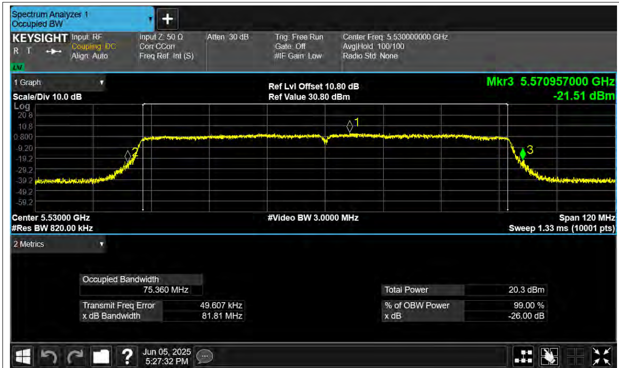
-26dB Bandwidth NVNT ac80 5530MHz Ant4
