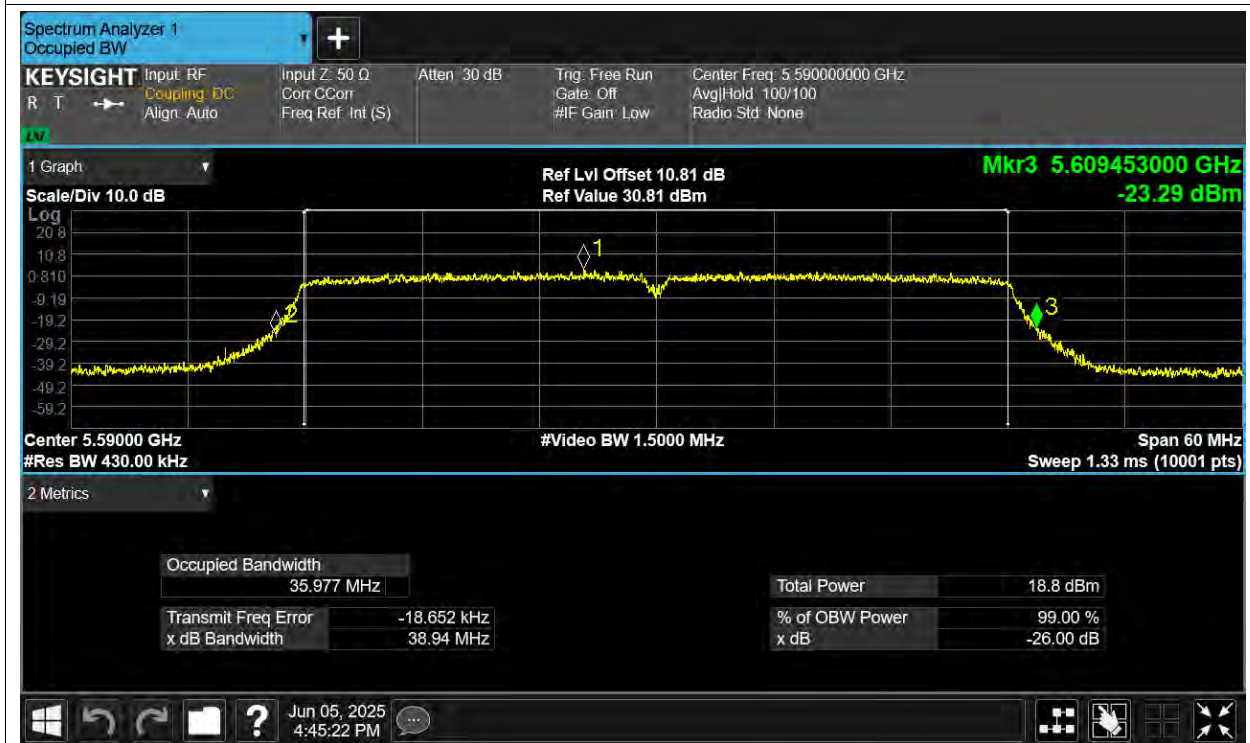
-26dB Bandwidth NVNT n40 5590MHz Ant3
