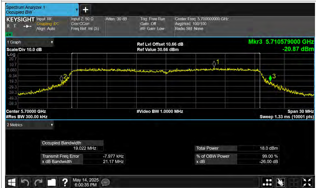
-26dB Bandwidth NVNT ax20 5700MHz Ant3
