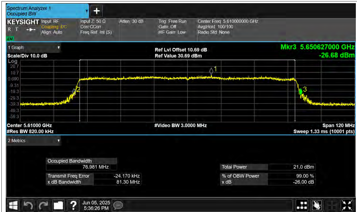
-26dB Bandwidth NVNT ax80 5610MHz Ant4
