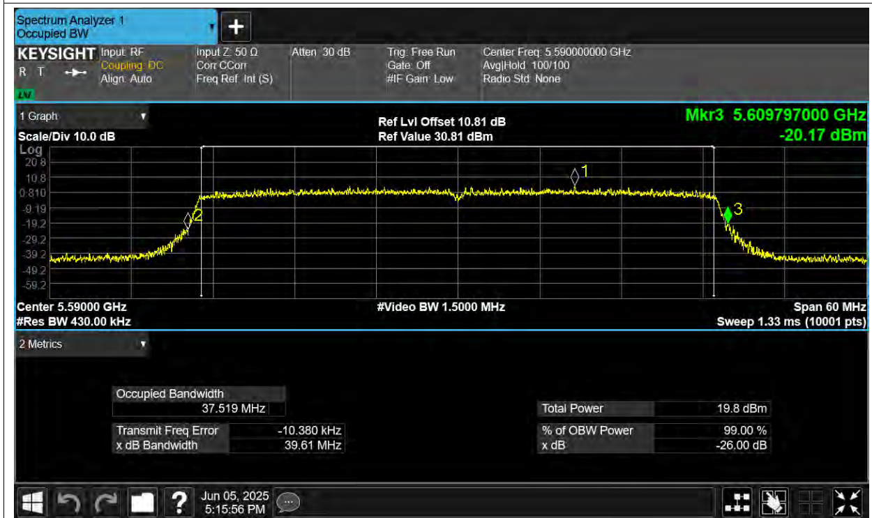
-26dB Bandwidth NVNT ax40 5590MHz Ant3
