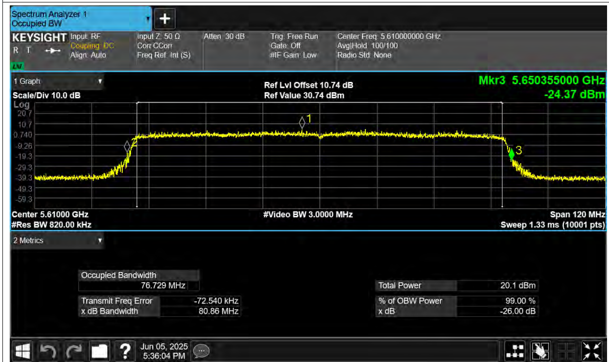
-26dB Bandwidth NVNT ax80 5610MHz Ant3
