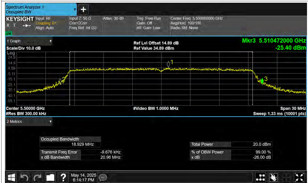
-26dB Bandwidth NVNT ax20 5600MHz Ant1
