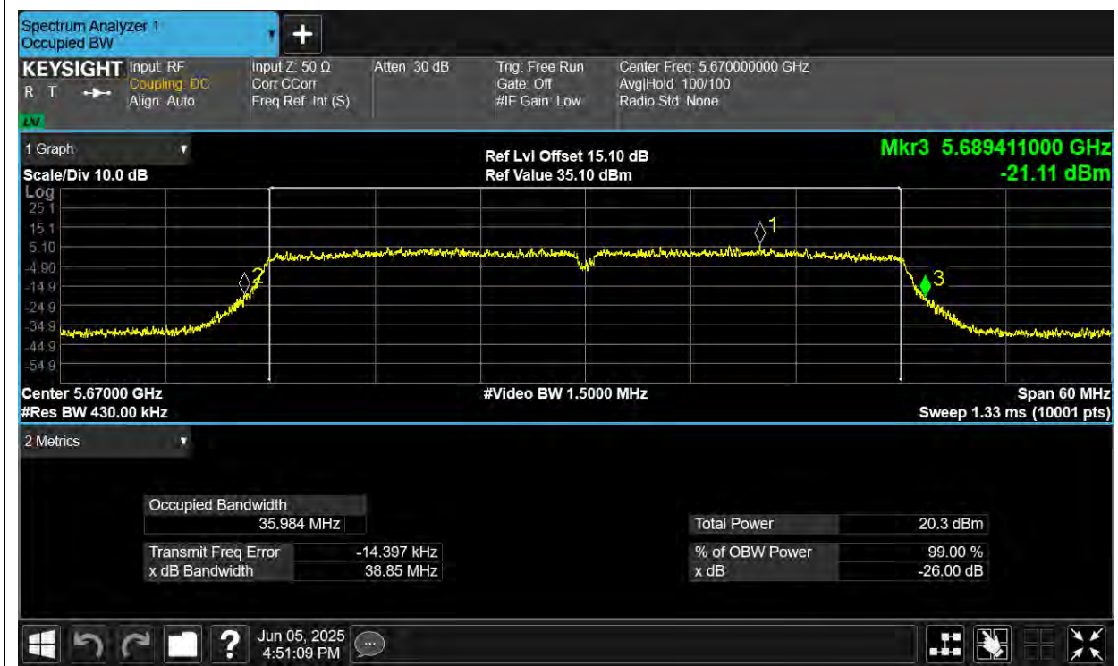
-26dB Bandwidth NVNT n40 5670MHz Ant4
