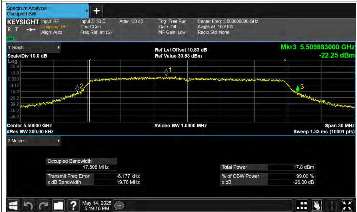
-26dB Bandwidth NVNT n20 5500MHz Ant3
