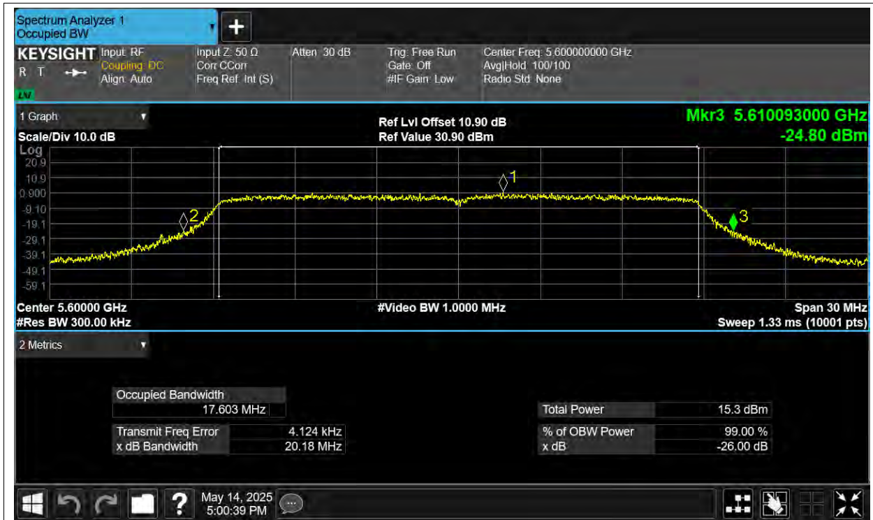
-26dB Bandwidth NVNT n20 5600MHz Ant2
