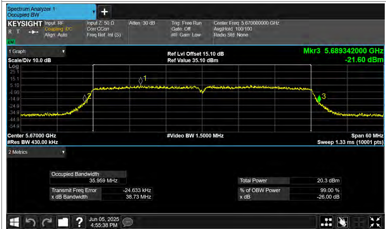
-26dB Bandwidth NVNT ac80 5530MHz Ant1
