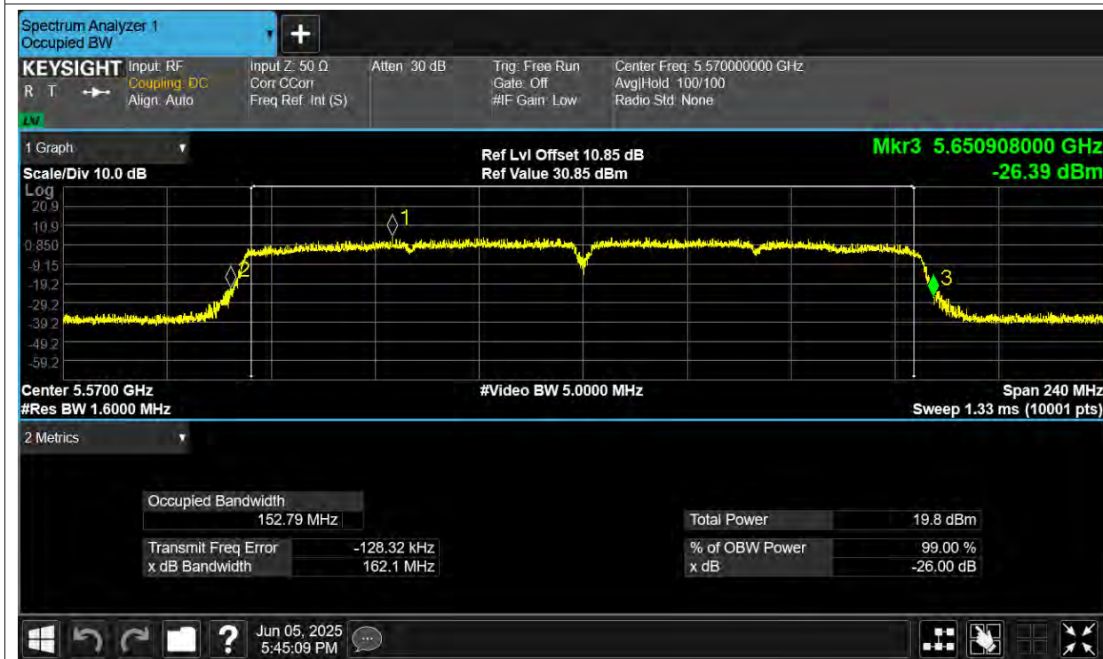
-26dB Bandwidth NVNT ac160 5570MHz Ant3
