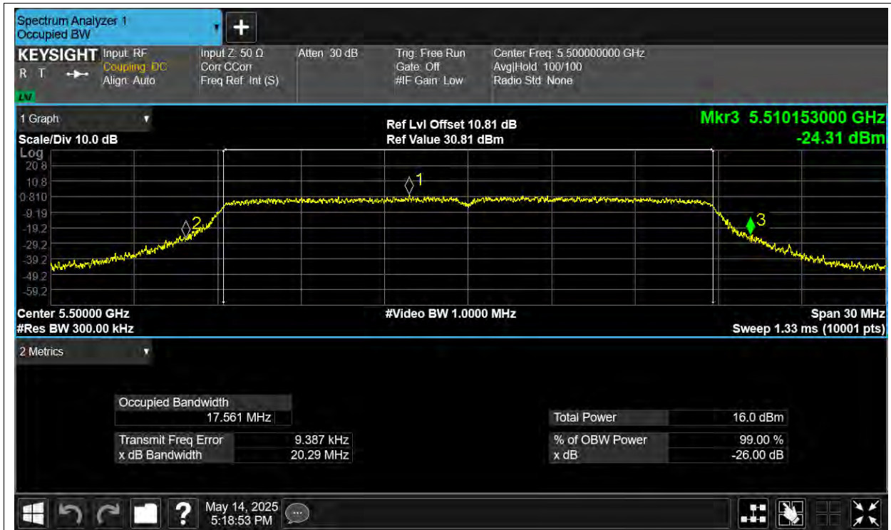
-26dB Bandwidth NVNT n20 5500MHz Ant2
