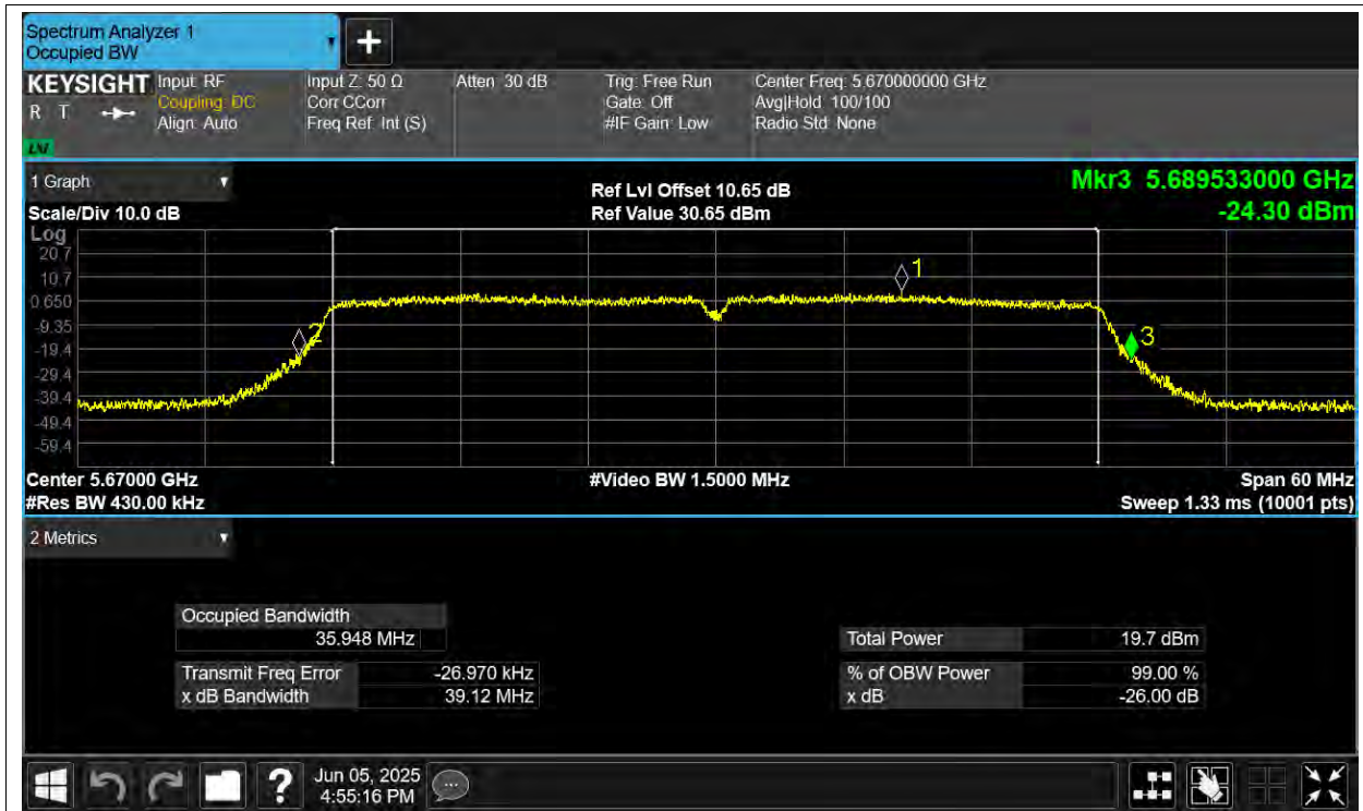
-26dB Bandwidth NVNT ac40 5670MHz Ant4
