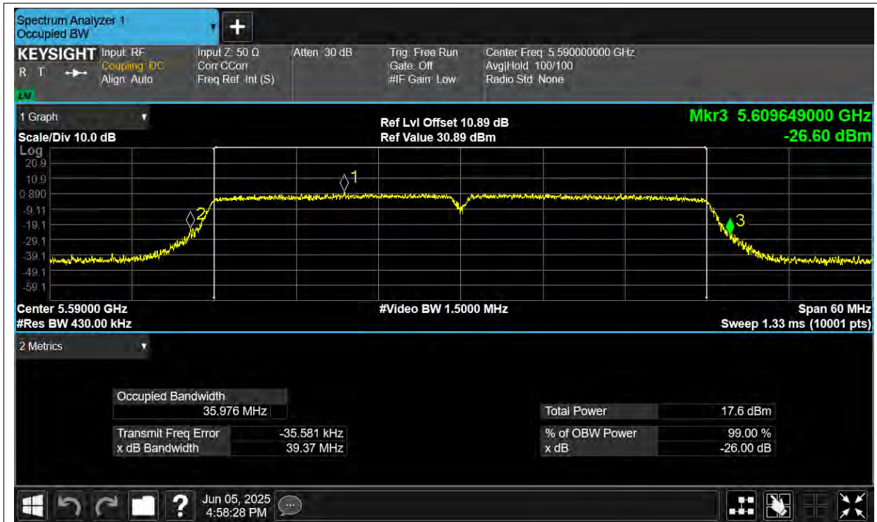
-26dB Bandwidth NVNT ac40 5590MHz Ant2
