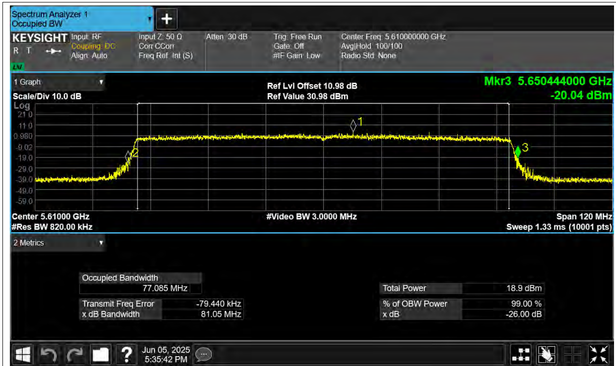
-26dB Bandwidth NVNT ax80 5610MHz Ant2
