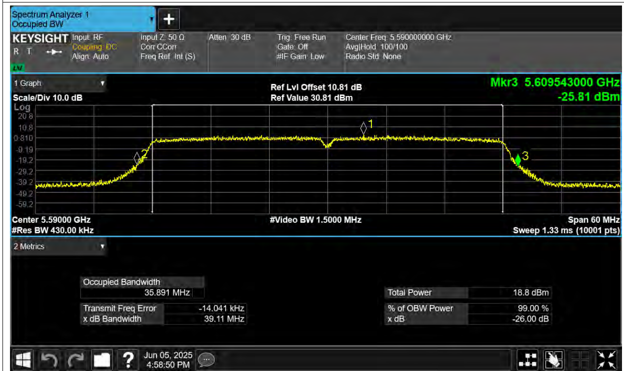
-26dB Bandwidth NVNT ac40 5590MHz Ant3
