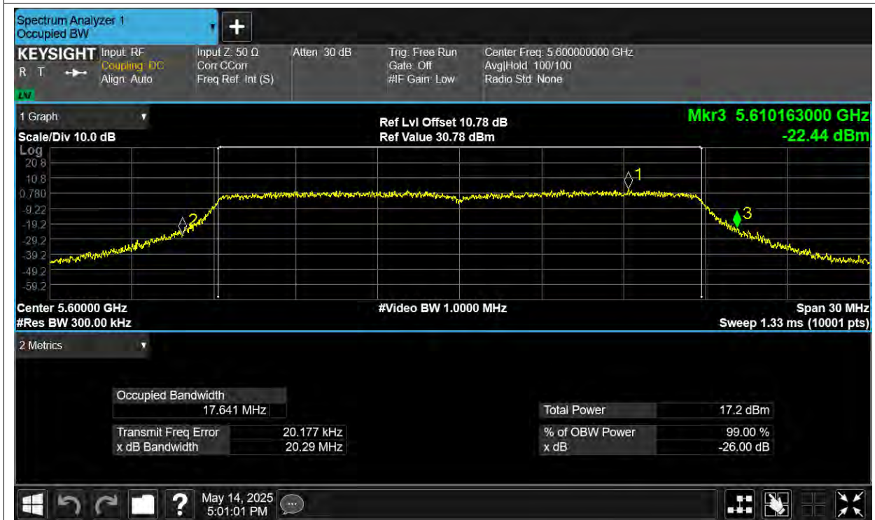
-26dB Bandwidth NVNT n20 5600MHz Ant3
