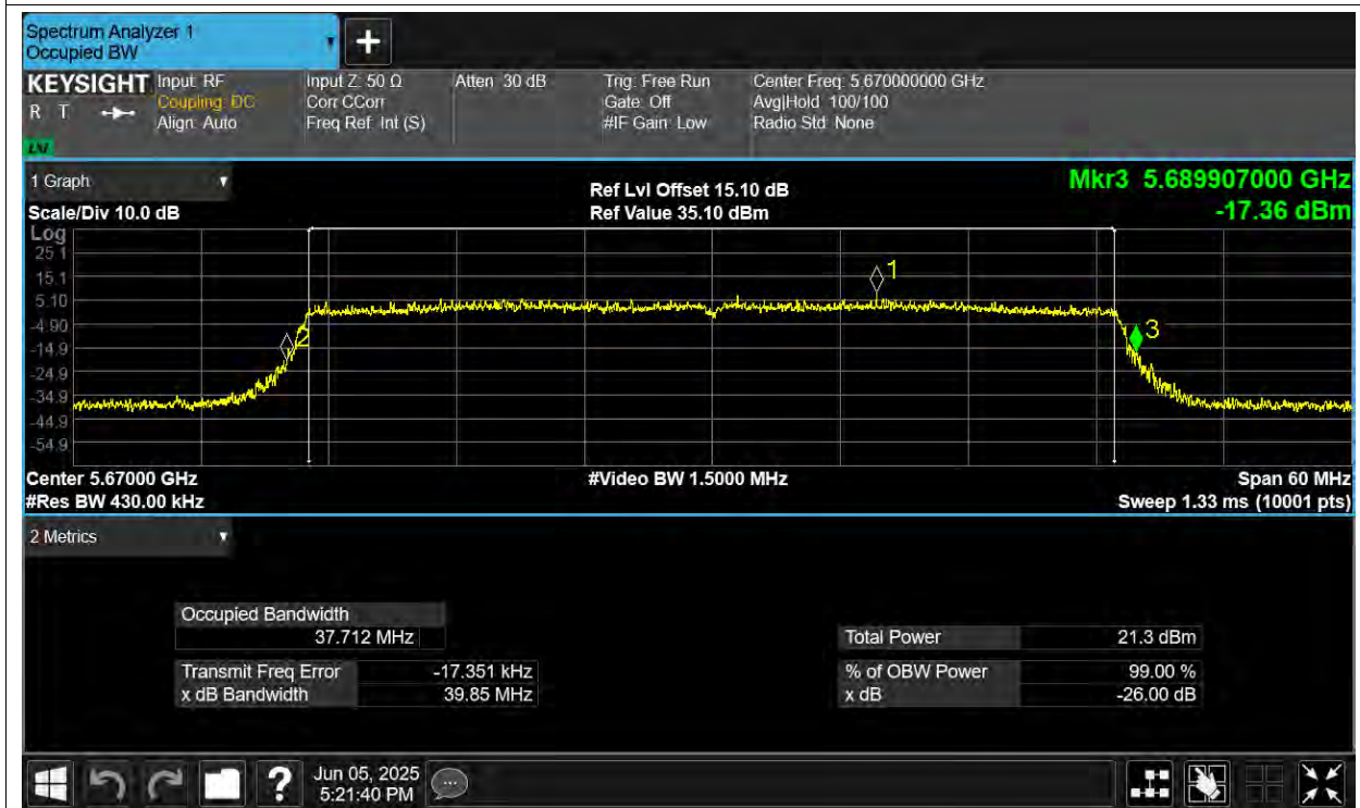
-26dB Bandwidth NVNT ax80 5530MHz Ant1
