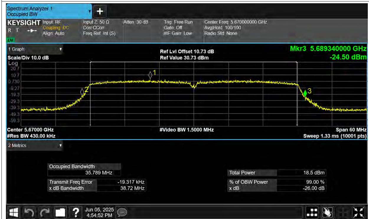
-26dB Bandwidth NVNT ac40 5670MHz Ant3
