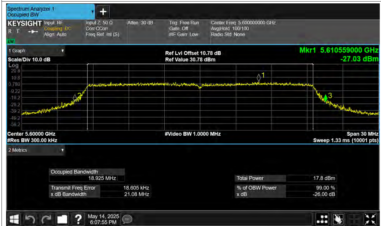
-26dB Bandwidth NVNT ax20 5600MHz Ant3
