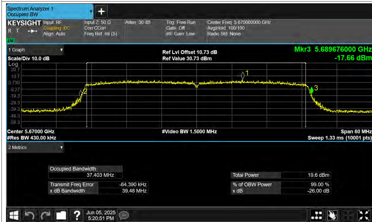
-26dB Bandwidth NVNT ax40 5670MHz Ant3
