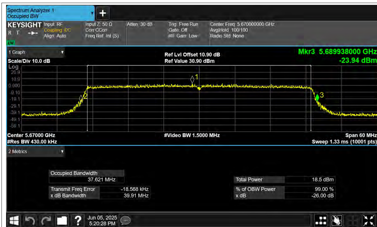
-26dB Bandwidth NVNT ax40 5670MHz Ant2
