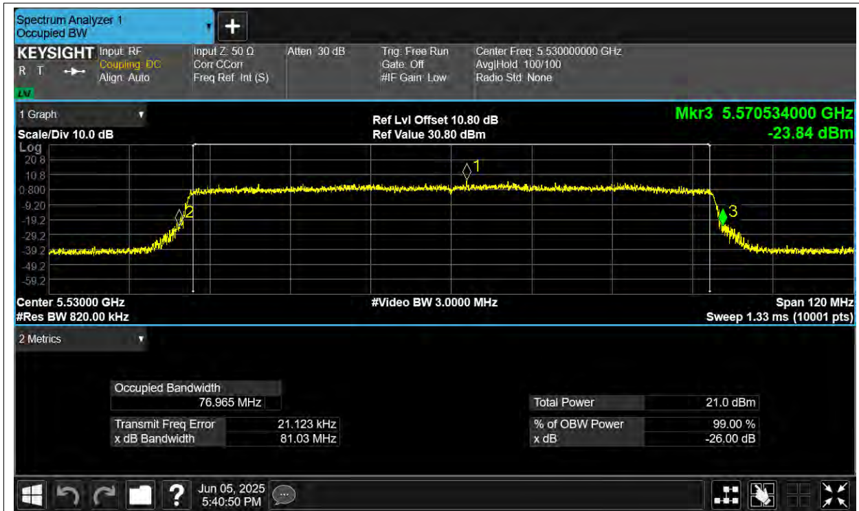
-26dB Bandwidth NVNT ax80 5530MHz Ant4
