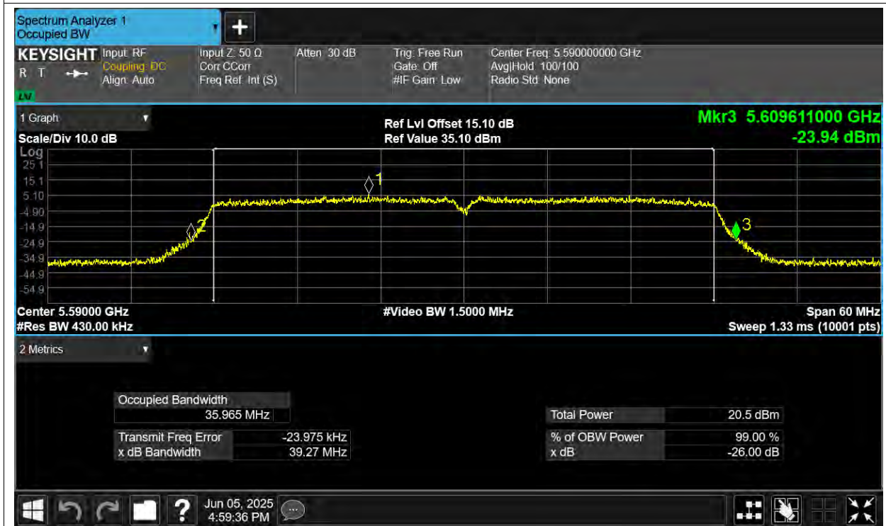
-26dB Bandwidth NVNT ac40 5670MHz Ant1
