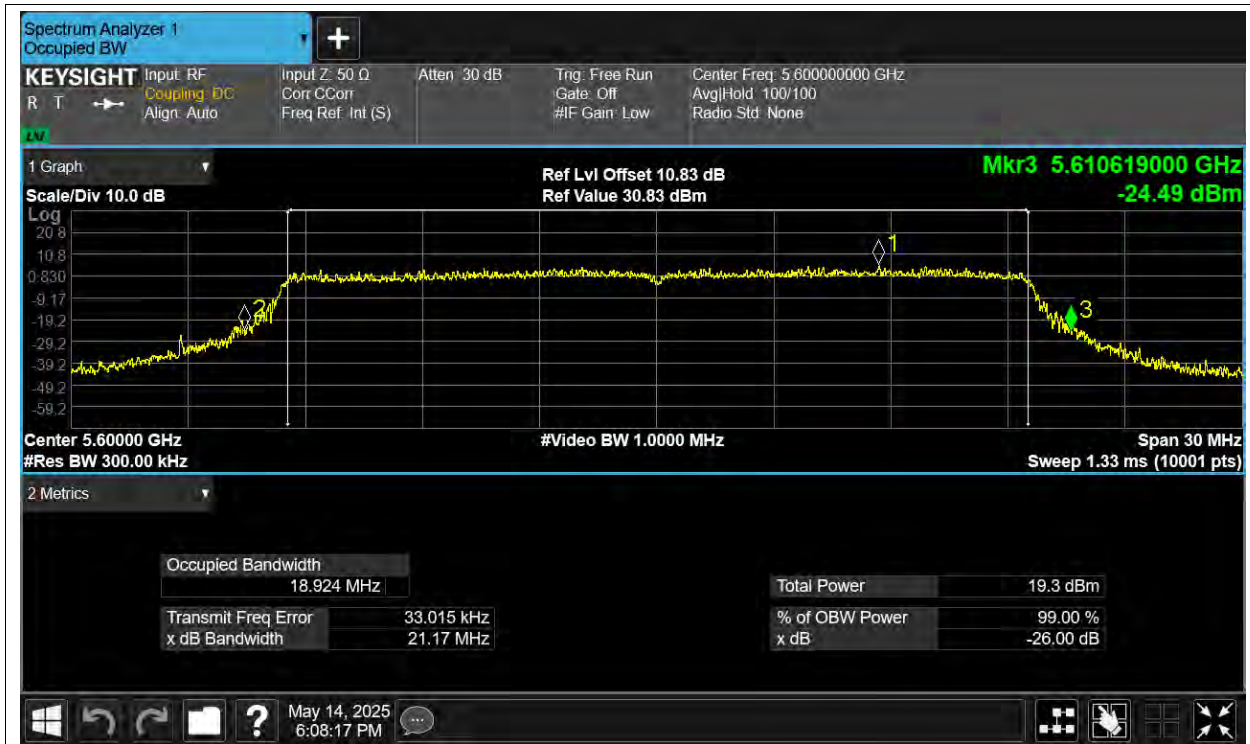
-26dB Bandwidth NVNT ax20 5600MHz Ant4
