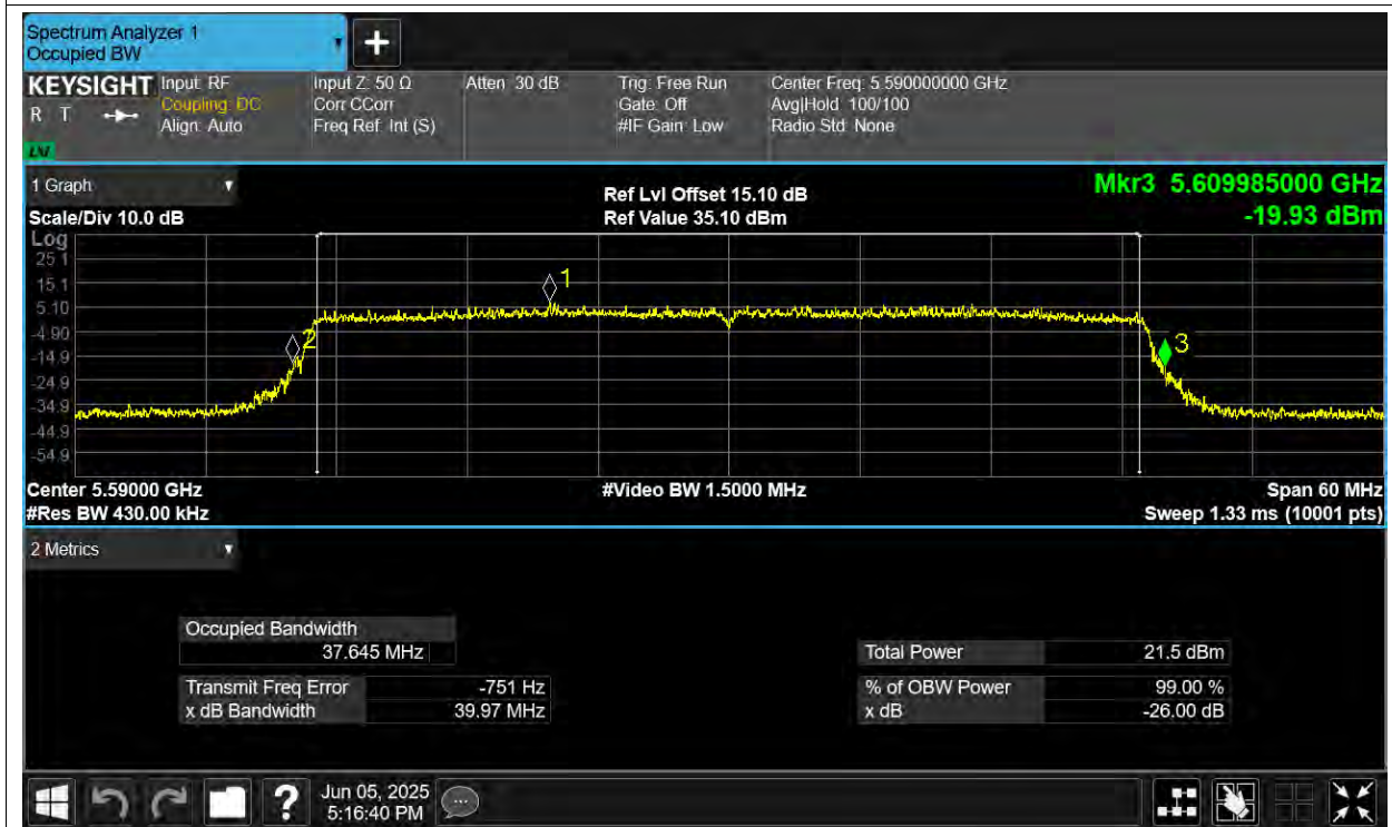
-26dB Bandwidth NVNT ax40 5670MHz Ant1
