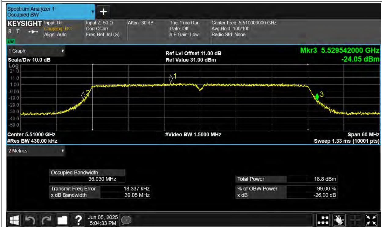
-26dB Bandwidth NVNT ac40 5510MHz Ant3
