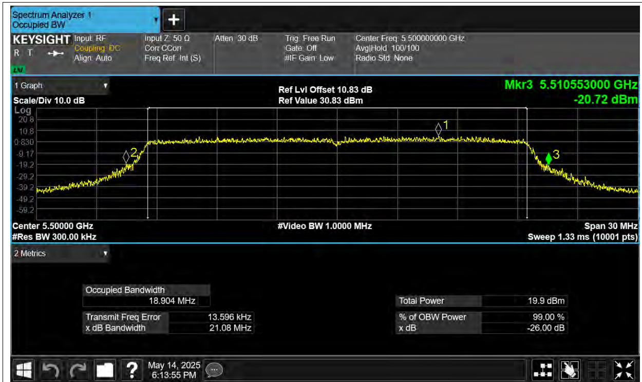
-26dB Bandwidth NVNT ax20 5500MHz Ant4
