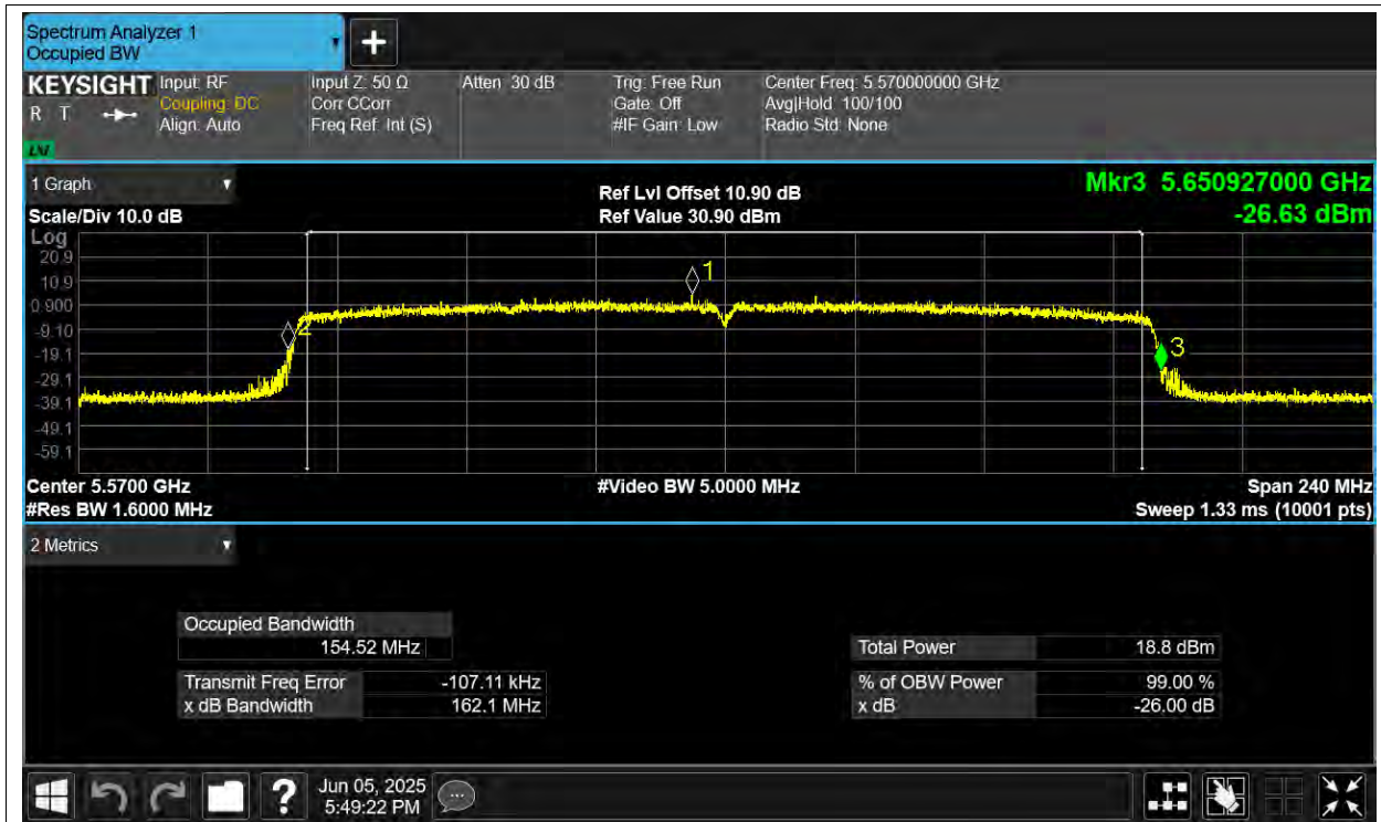
-26dB Bandwidth NVNT ax160 5570MHz Ant2
