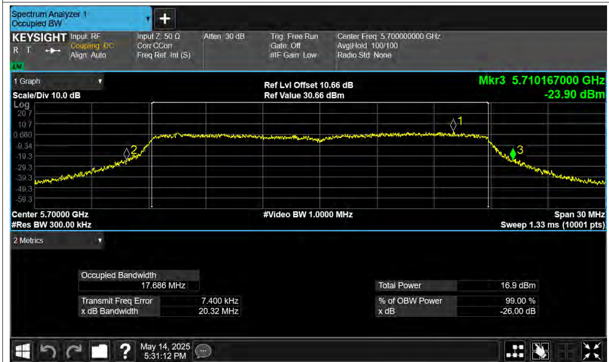
-26dB Bandwidth NVNT ac20 5700MHz Ant3
