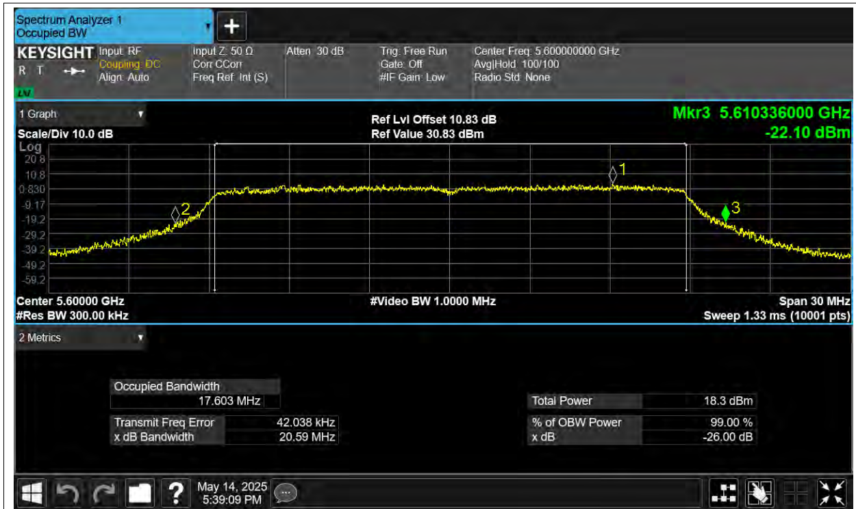
-26dB Bandwidth NVNT ac20 5600MHz Ant4
