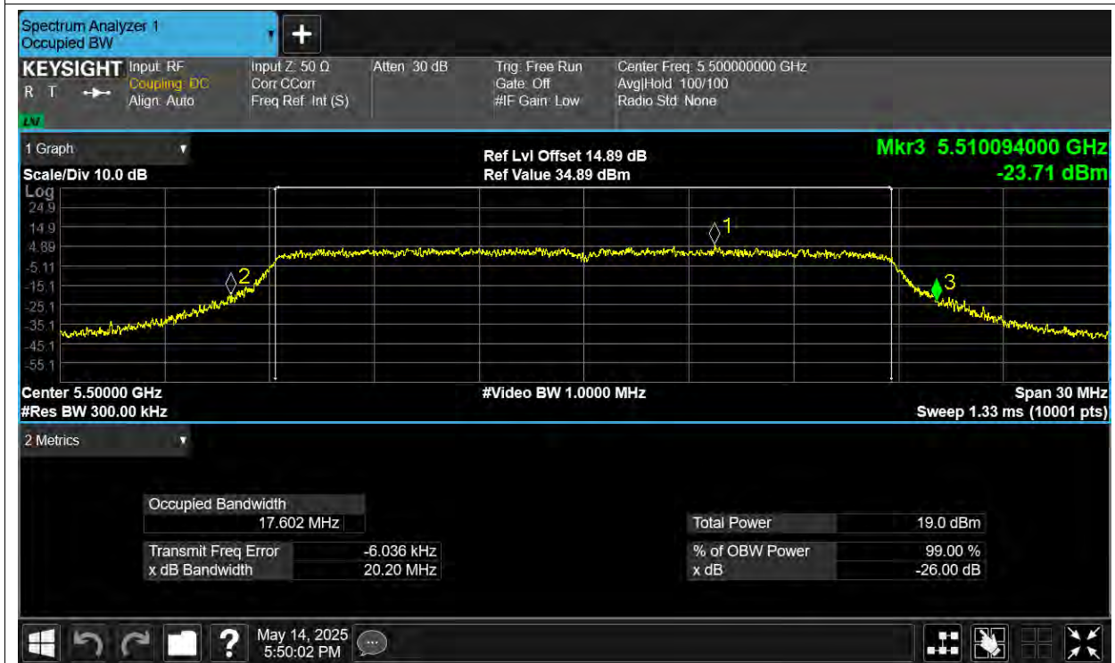
-26dB Bandwidth NVNT ac20 5600MHz Ant1
