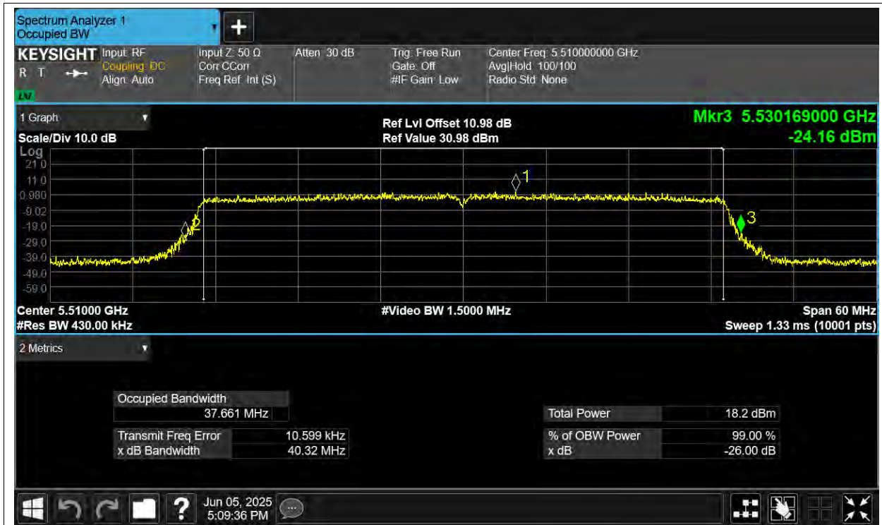
-26dB Bandwidth NVNT ax40 5510MHz Ant2
