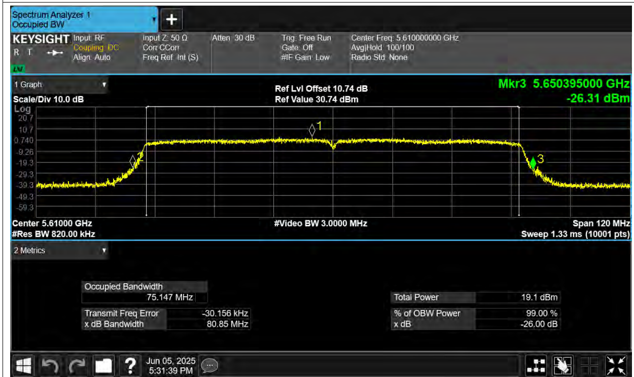
-26dB Bandwidth NVNT ac80 5610MHz Ant3
