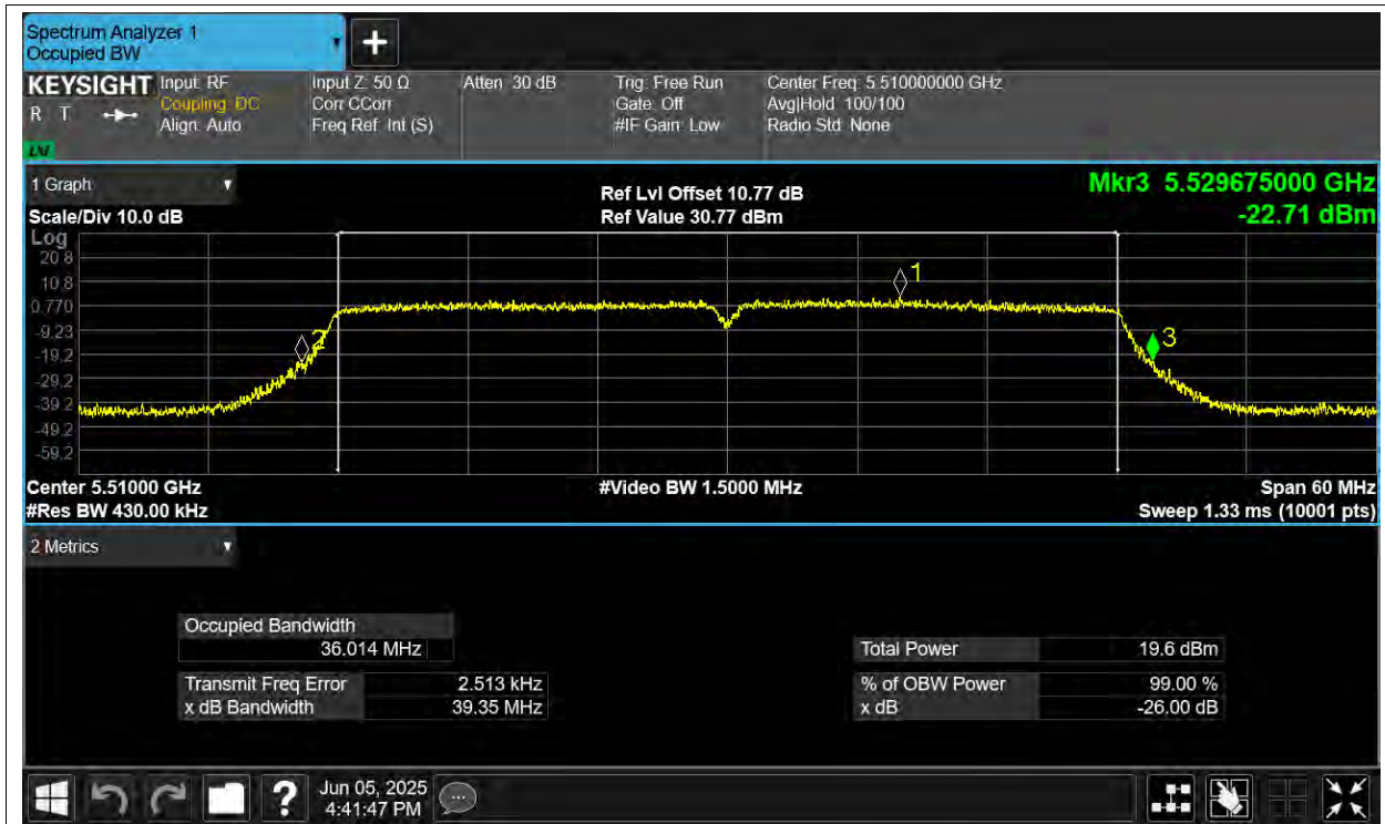
-26dB Bandwidth NVNT n40 5510MHz Ant4
