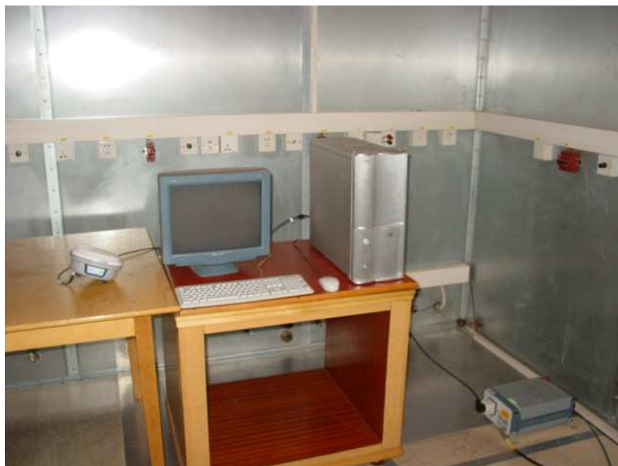
FCC CONDUCTED EMISSION TEST SETUP-Reading
