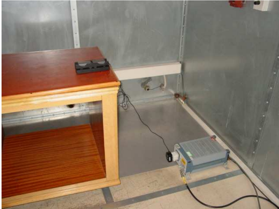
FCC CONDUCTED EMISSION TEST SETUP-Charging
