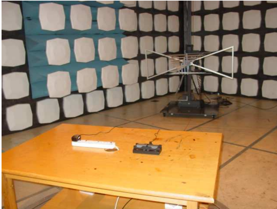
FCC RADIATED EMISSION TEST SETUP-Charging
