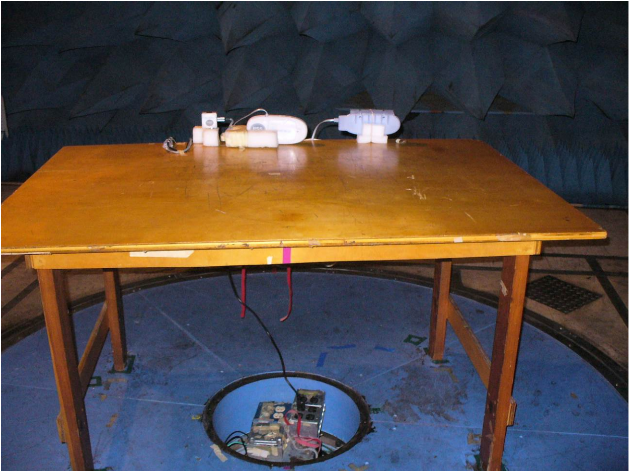
Figure 1: Radiated Emissions – Front View
