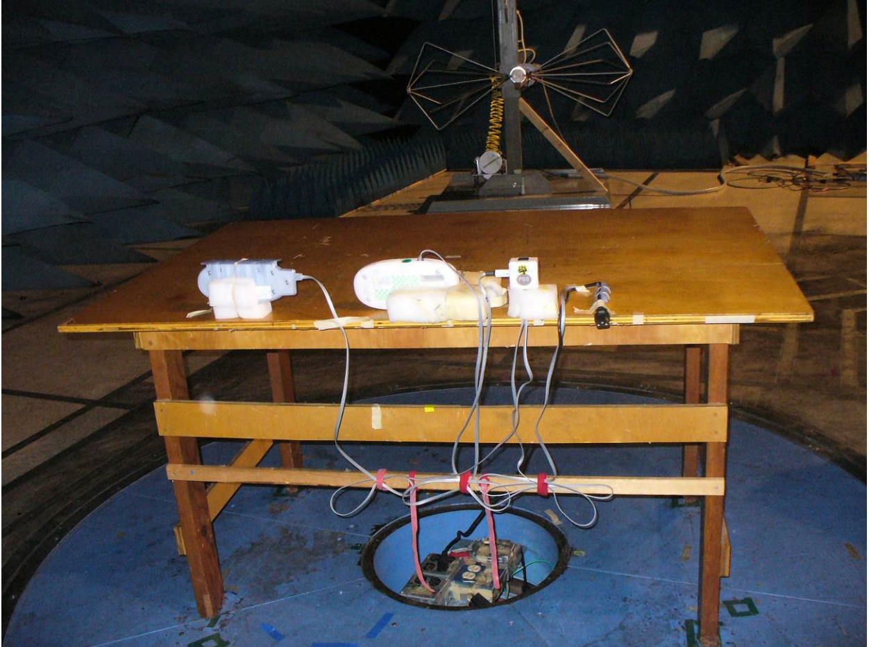
Figure 3: Radiated Emissions – Back View 30 MHz – 200 MHz
