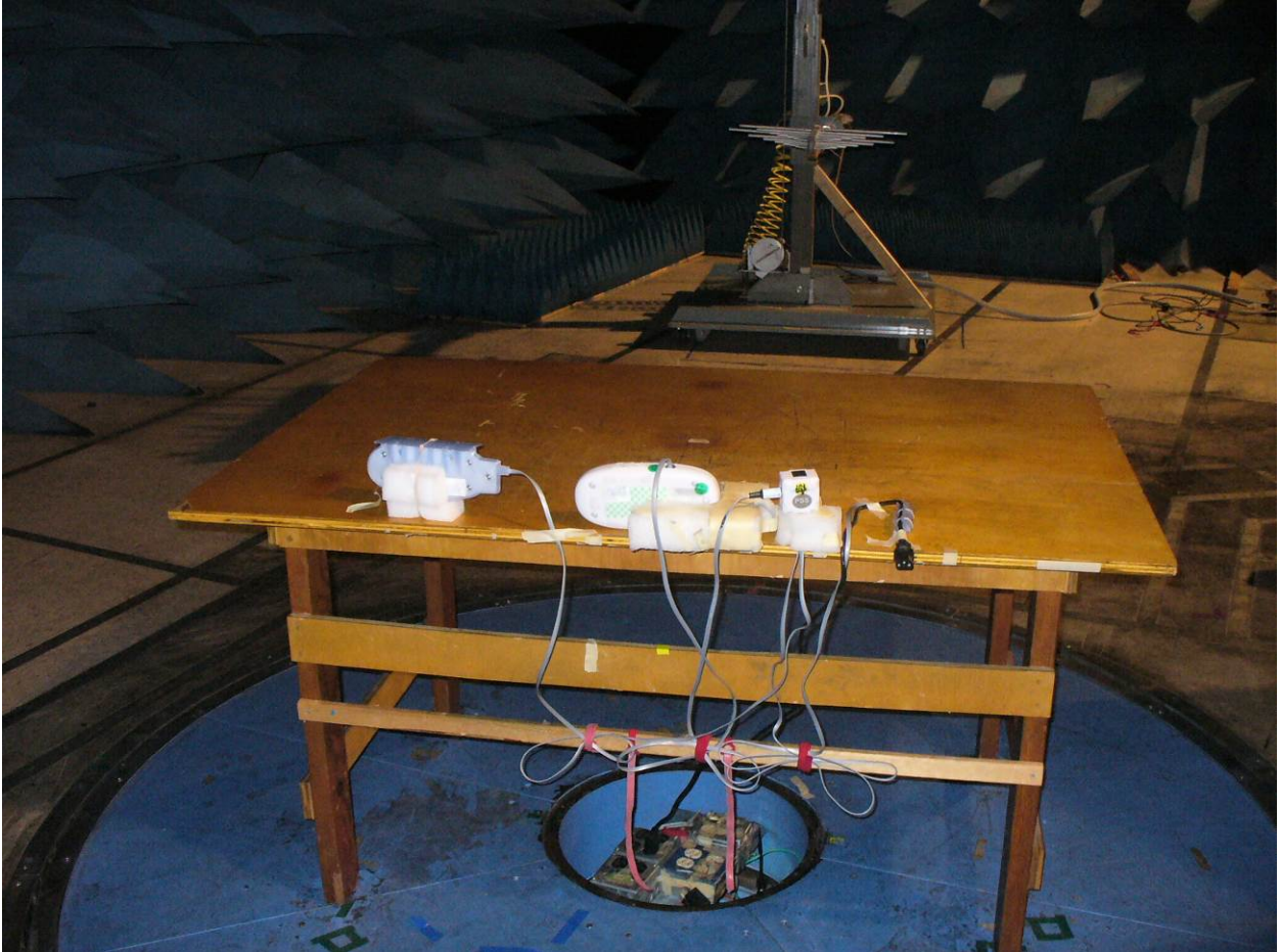
Figure 4: Radiated Emissions – Back View 200 MHz – 1 GHz
