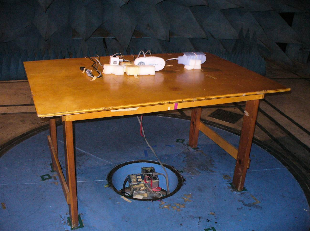
Figure 5: Radiated Emissions – Front View 1 GHz – 5 GHz
