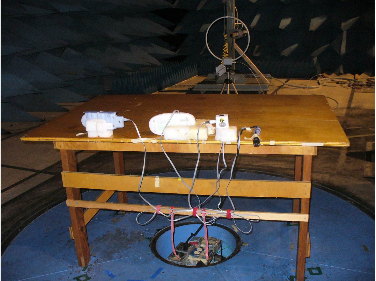
Figure 2: Radiated Emissions – Back View 10 kHz – 30 MHz
