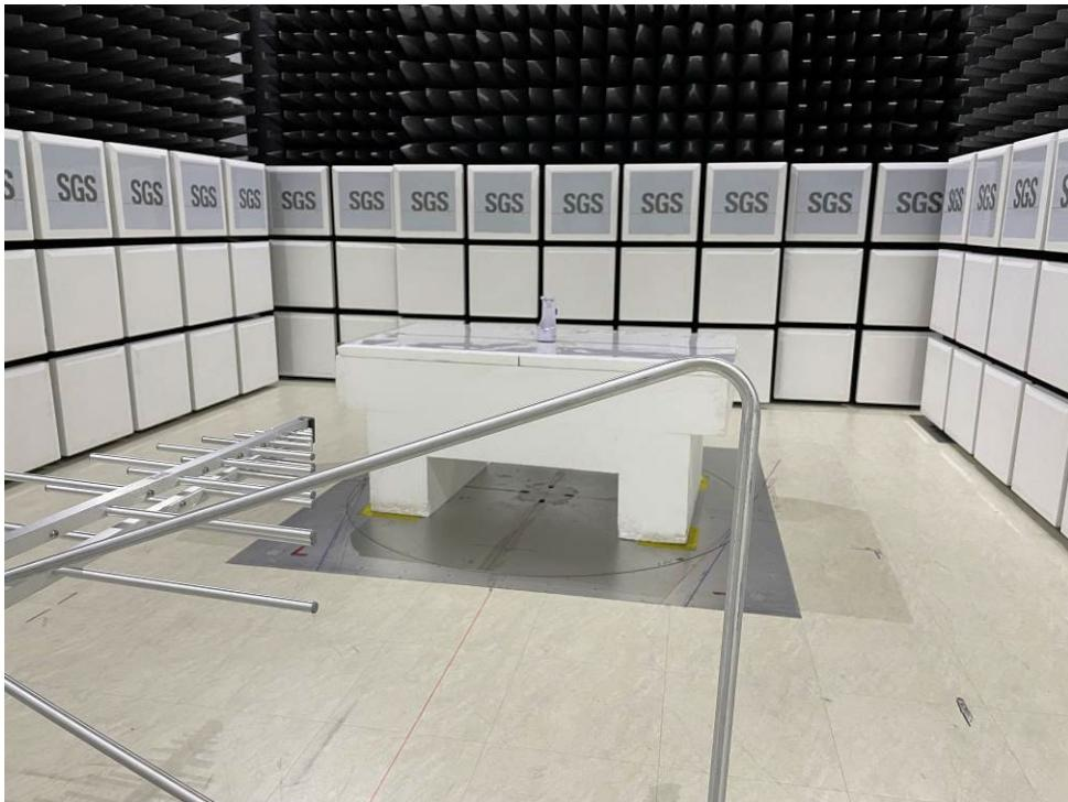
**Radiated Emissions (Above 1GHz) Test Setup**
