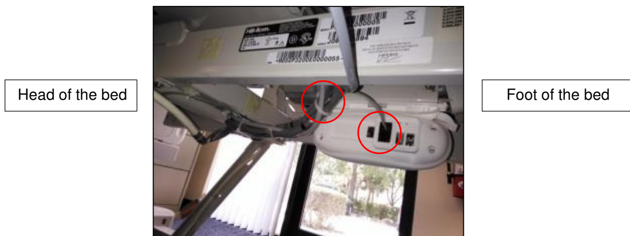
Figure 11. AC Line Power Sensor Cable Routing to Bed Beacon and Cable Tie Holder Placement
