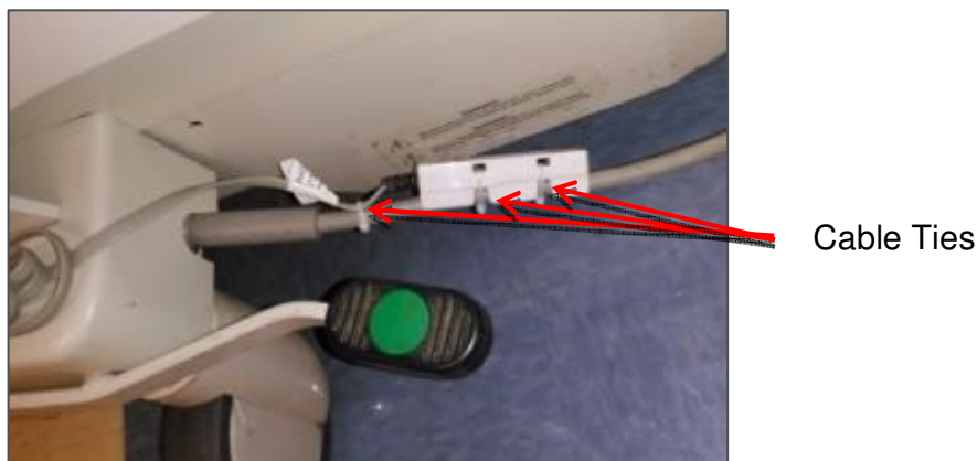
Figure 5. AC Line Power Sensor Cable Routing to the Bed Beacon
