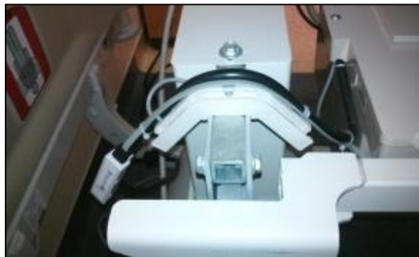
Figure 4. AC Line Power Sensor Cable Routing to the Bed Beacon
