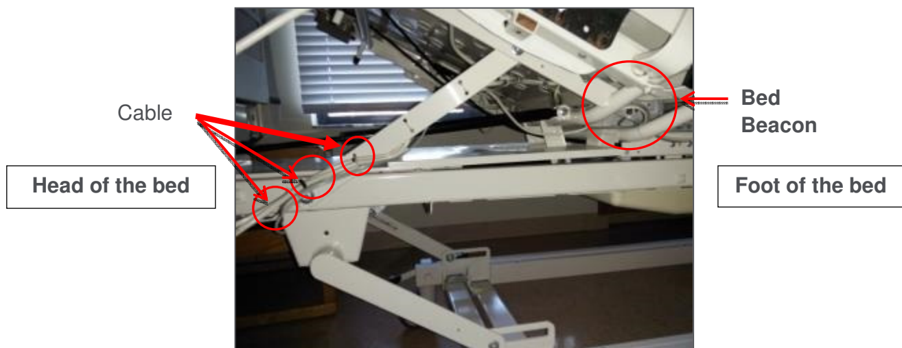
Figure 5. AC Line Power Sensor Cable Routing
