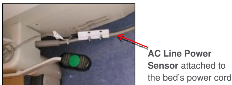
Figure 3. The AC Line Power Sensor Installation Location on the Bed
