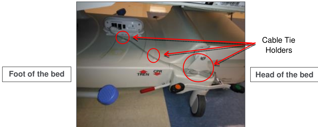
Figure 6. AC Line Power Sensor Cable Routing
