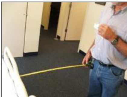
Figure 14. Test Badge Activation Distance from Bed's Handrail Center is 18" (at edge for stretcher installations)
