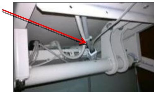
Figure 2. The AC Line Power Sensor Installation Location on the Bed
