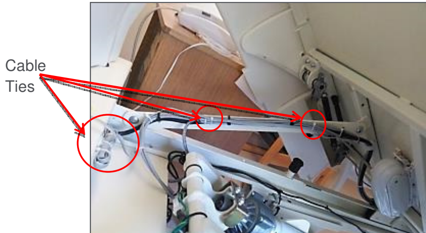
Figure 5. AC Line Power Sensor Cable Routing
