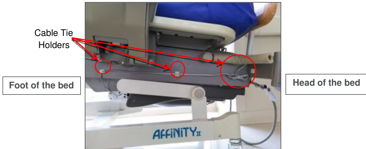
Figure 5. AC Line Power Sensor Cable Routing
