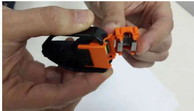
Figure 5. Press the opener to release the cover.
