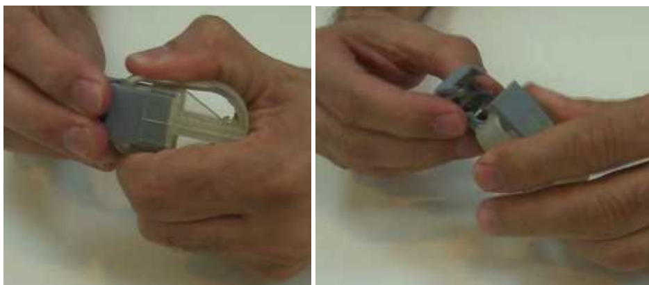
Figure 6. Press the opener to release the cover.
