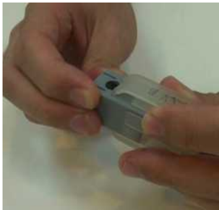
Figure 5. Snap the opener into the sensor holes.
