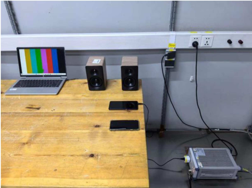
Photograph 1: Set-up for Conducted Emission on AC Mains
