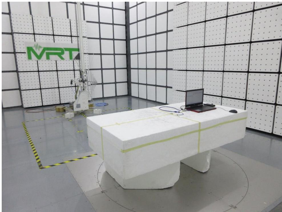
Description: Radiated Emission Test Setup for above 1GHz – Left Ear
