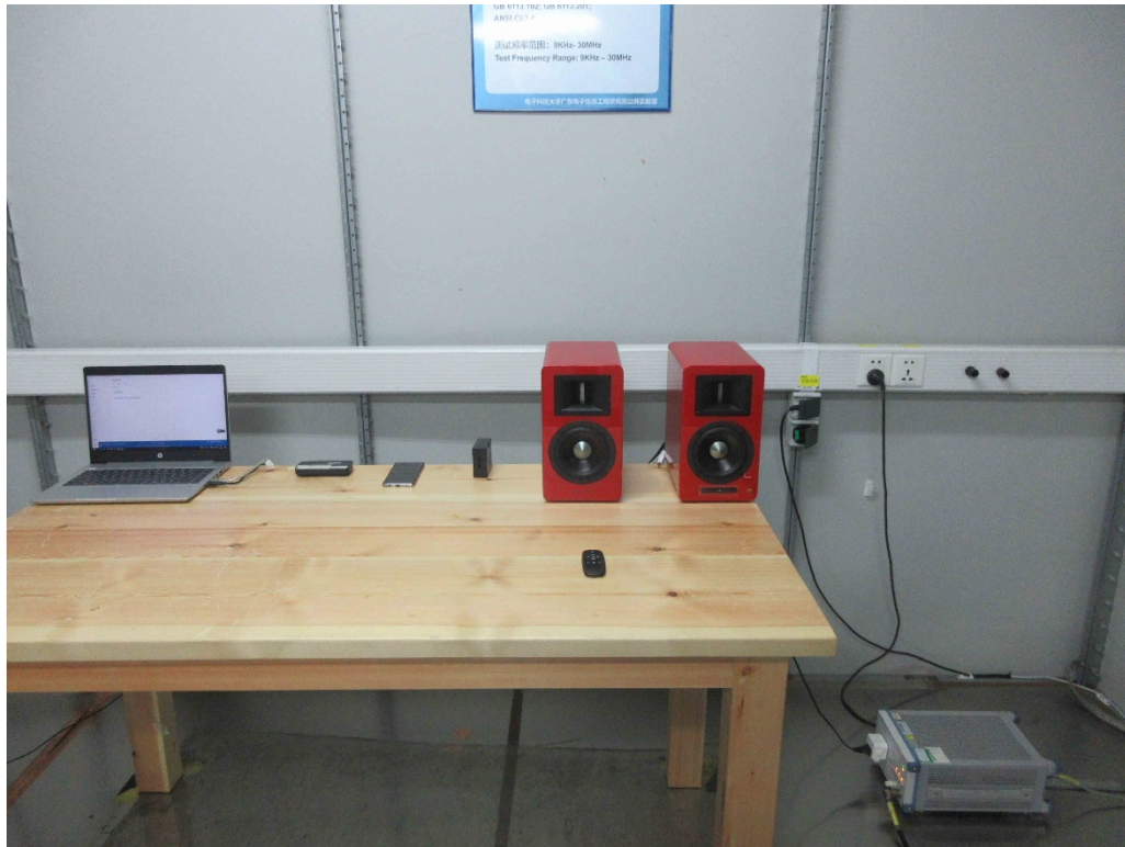
Photograph 1: Set-up for Conducted Emission on AC Mains
