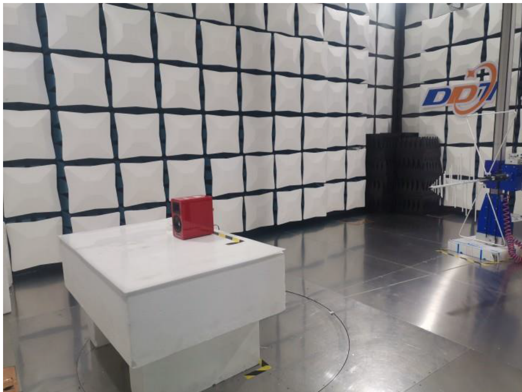
Photograph 2: Set-up for Radiated Spurious Emission, below 1GHz
