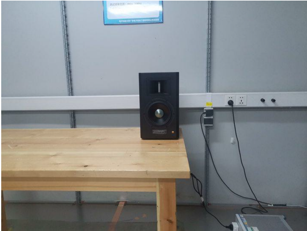
Photograph 1: Set-up for Conducted Emission on AC Mains
