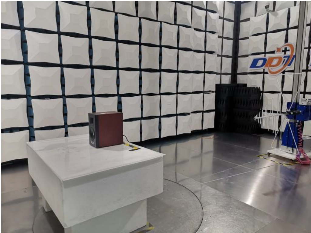
Photograph 2: Set-up for Radiated Spurious Emission, below 1GHz
