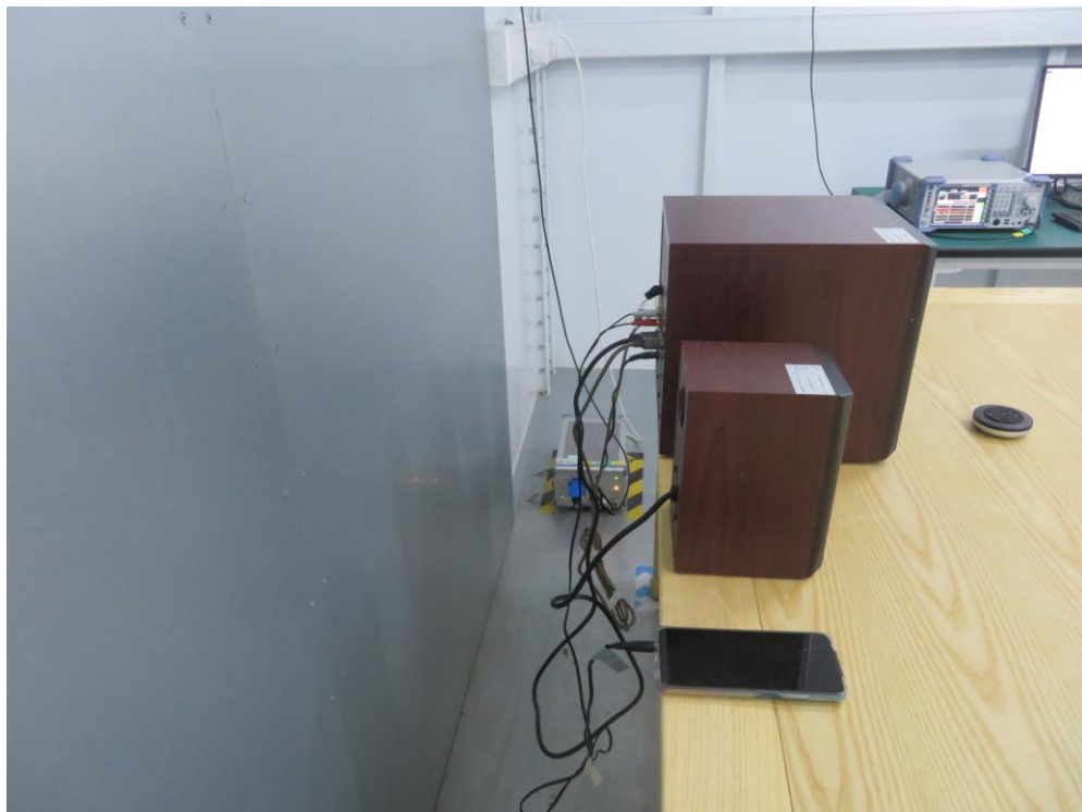
Description: Back View of AC Conducted Emission Test Setup
