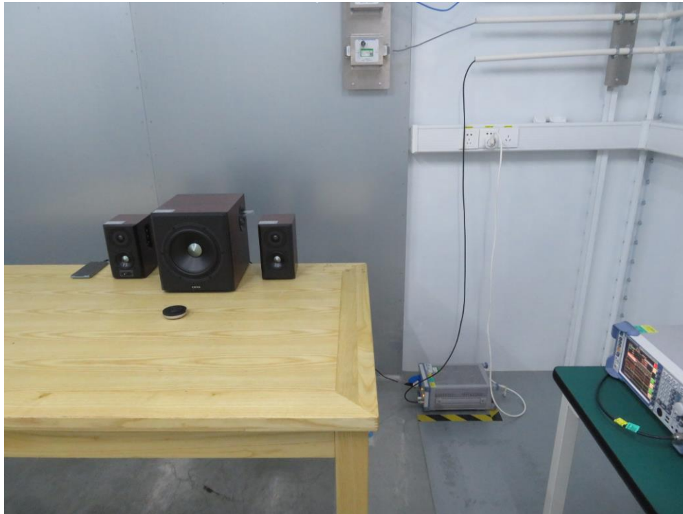
Description: Back View of AC Conducted Emission Test Setup
