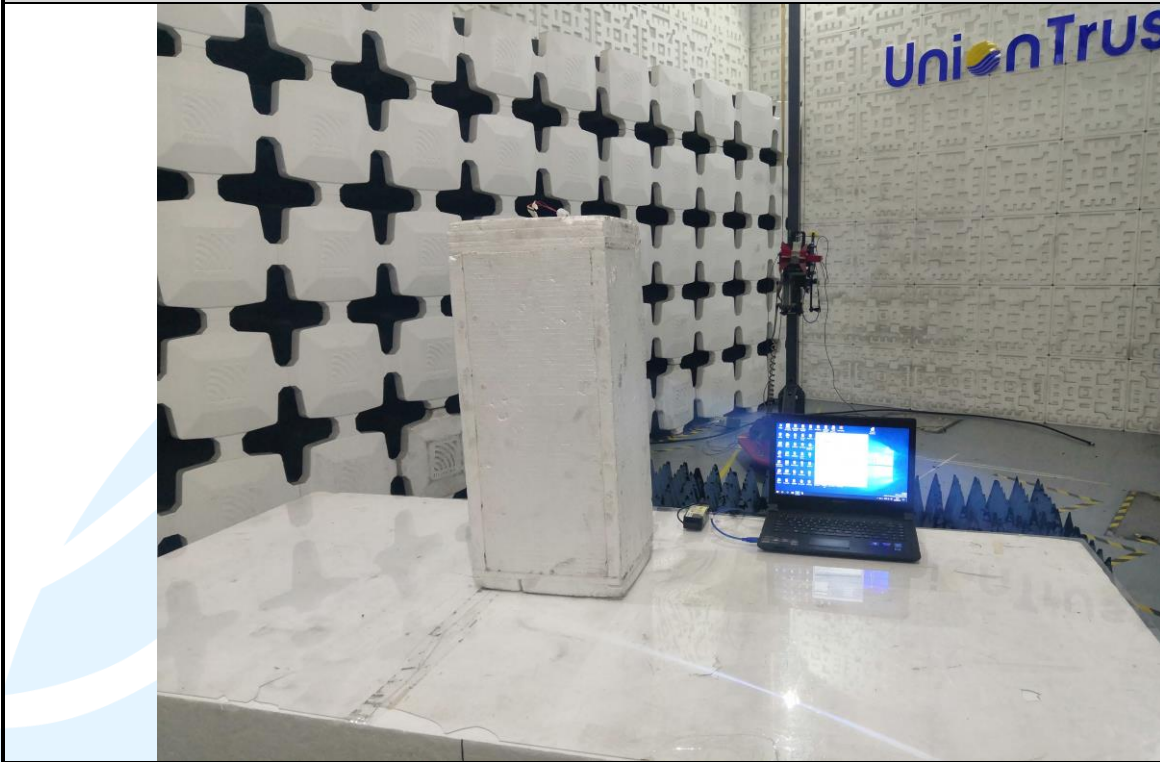
Radiated emission Test Setup (Above 1 GHz) -Left
