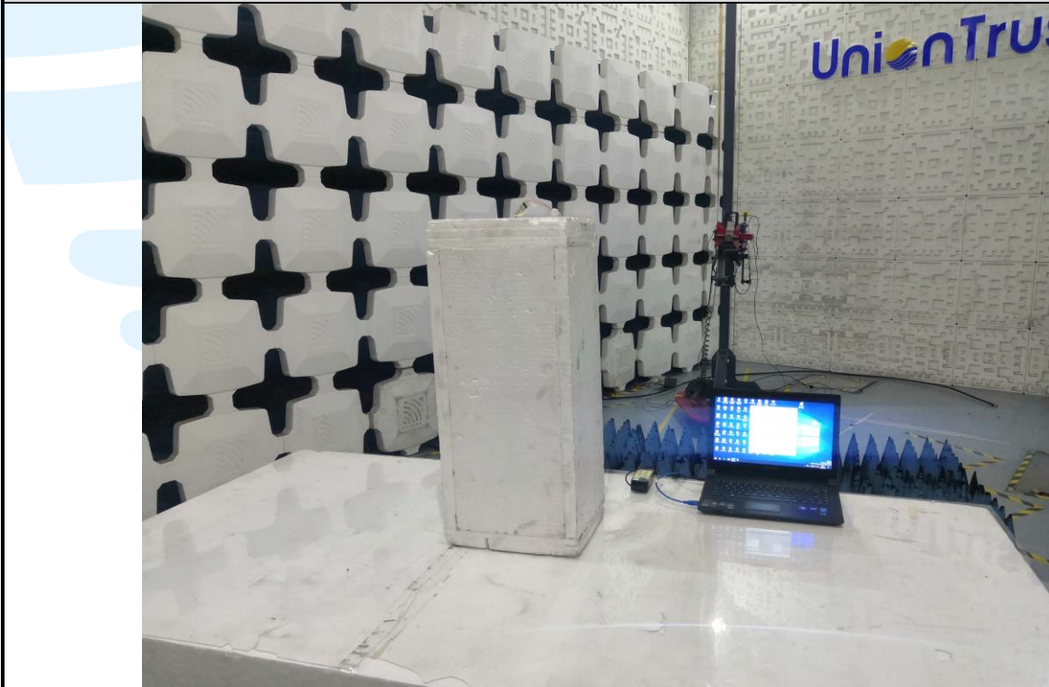
Radiated emission Test Setup (Above 1 GHz) -Right
