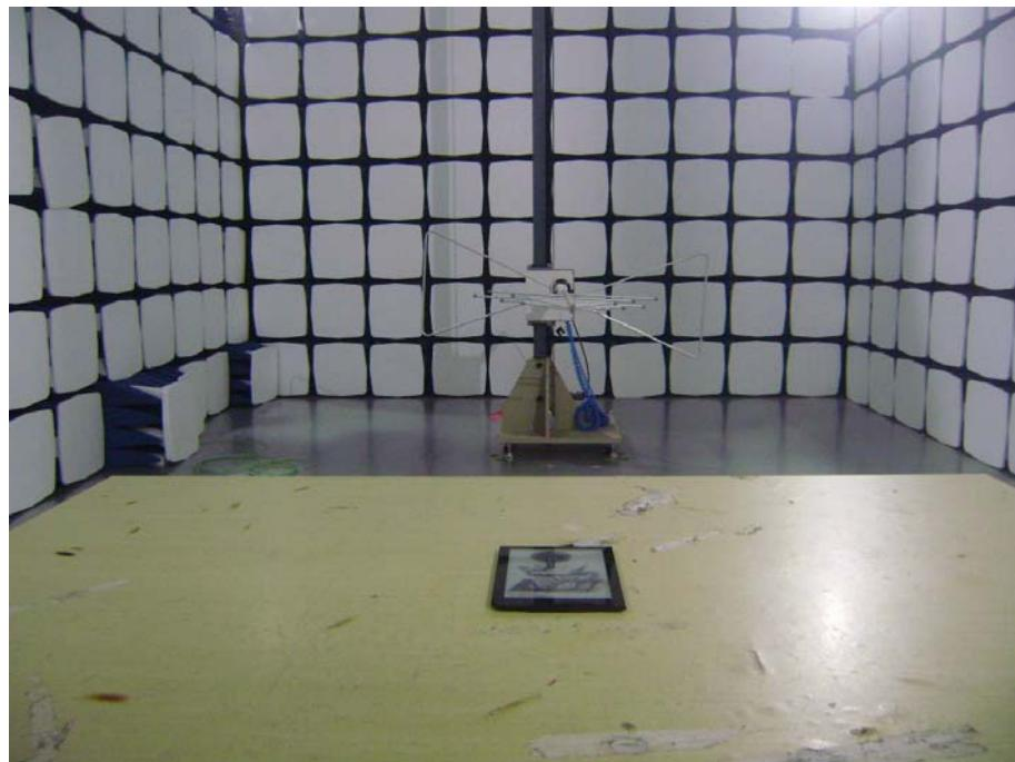
**Radiation Emission Test Setup (Above 1GHz)**
