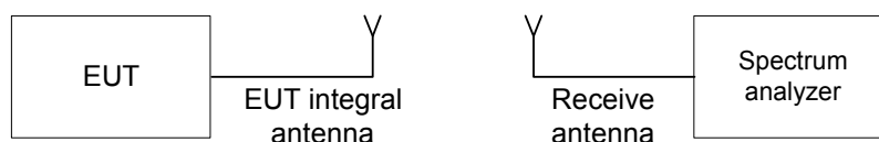
Figure 7.1.1 Setup for transmitter shut down test
