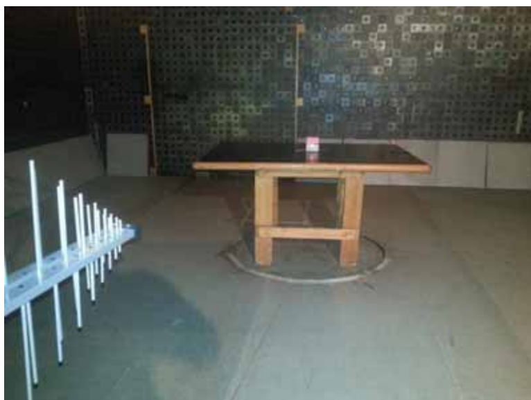
Photograph 8.1.1 Setup for radiated emission measurements
