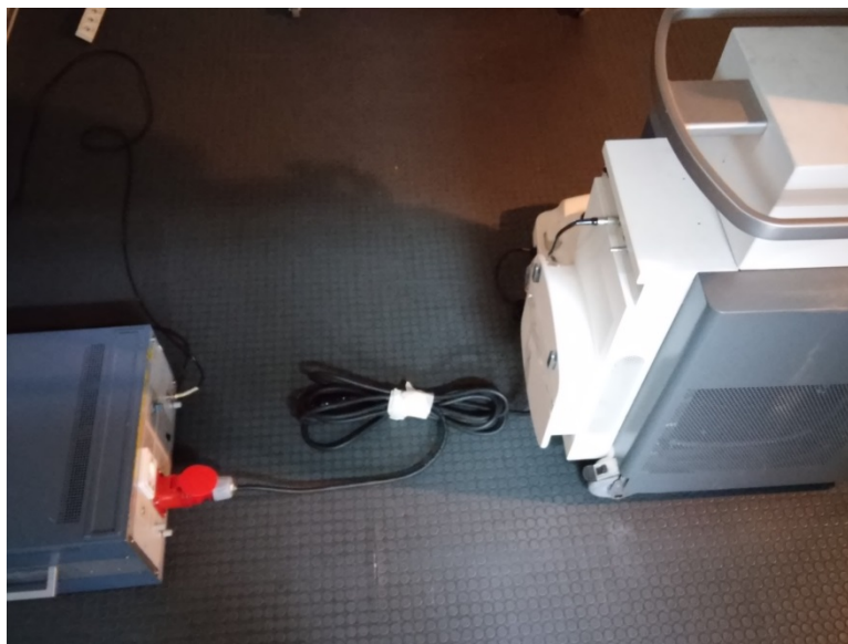
Photograph 8.1.1 Setup for conducted emission measurements
