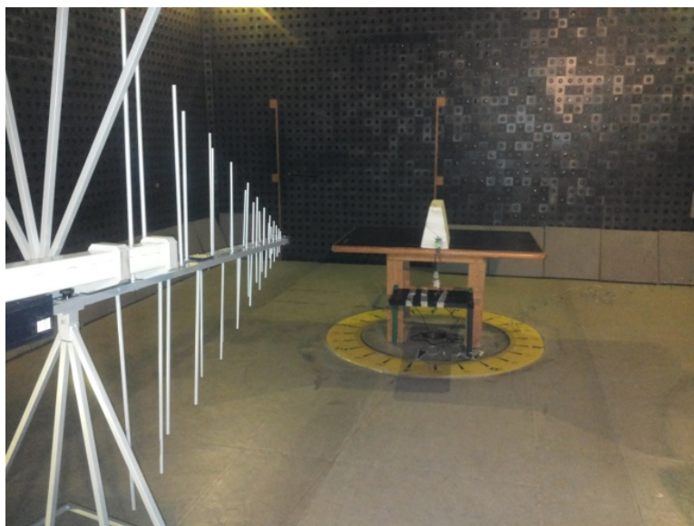
Photograph 8.2.2 Setup for radiated emission measurements, EUT cabling
