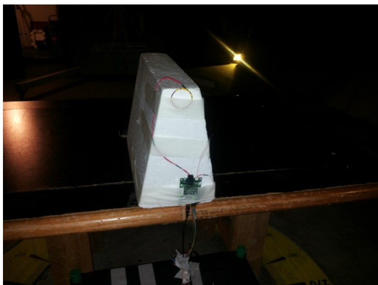
Photograph 8.2.2 Setup for radiated emission measurements, EUT cabling
