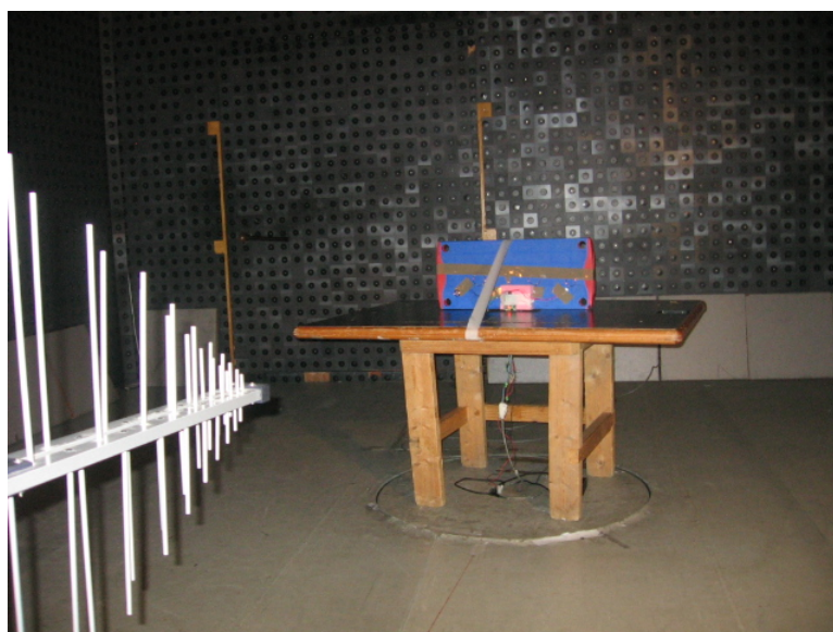
Photograph 8.1.1 Setup for preliminary radiated emission measurements
