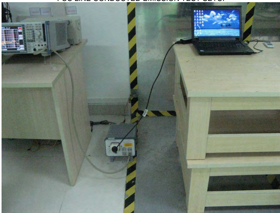
FCC LINE CONDUCTED EMISSION TEST SETUP
