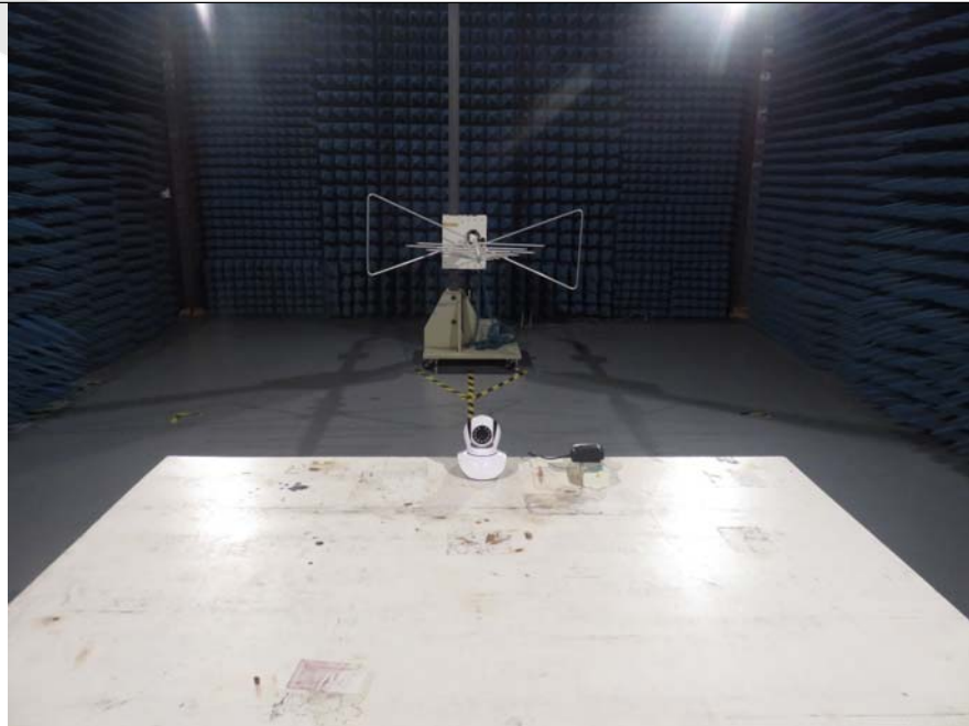
6.2.Photo of Radiation Emission Test
