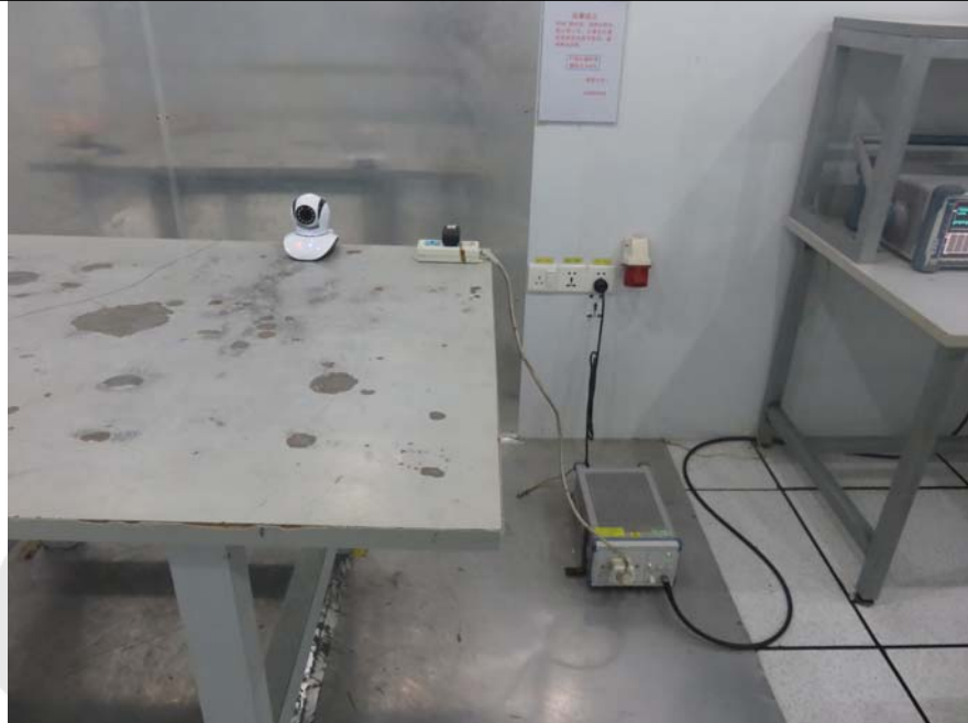
6.1.Photo of Conducted Emission Measurement
