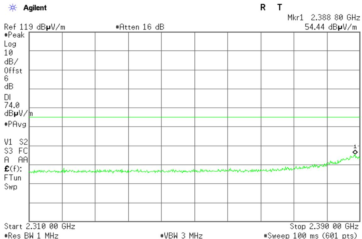
**Detector mode: Average****Polarity: Horizontal**
