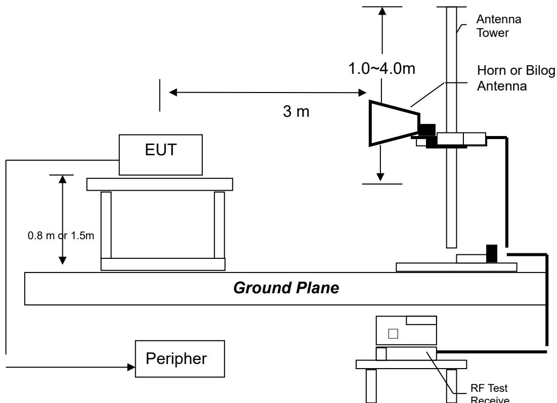
Radiated emission measurements were performed from 9KHz to tenth harmonic or 40GHz.
