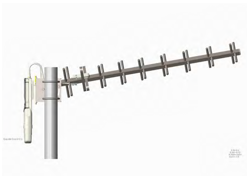
Figure 152: Yagi antenna alignment - upward tilt
