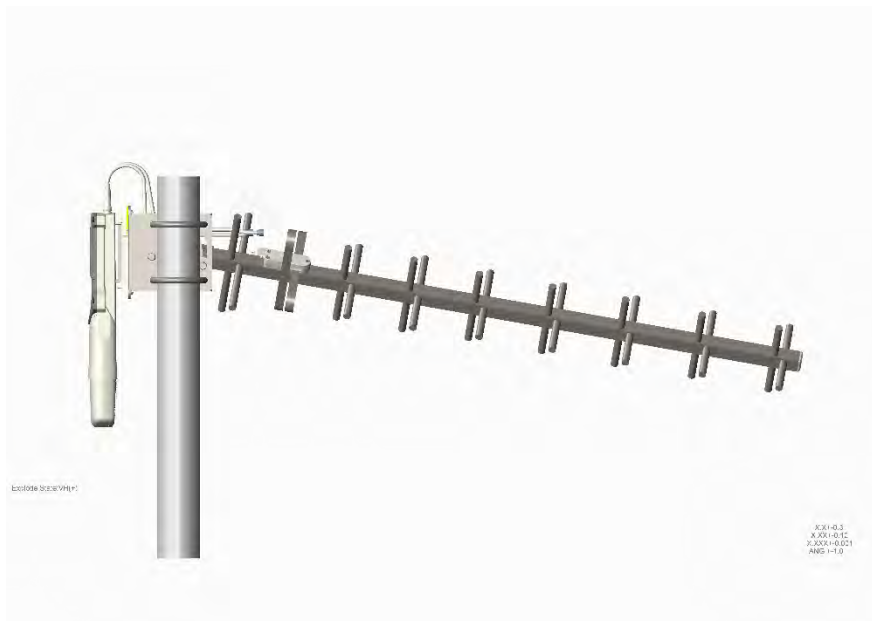
Figure 153: Yagi antenna alignment - downward tilt
