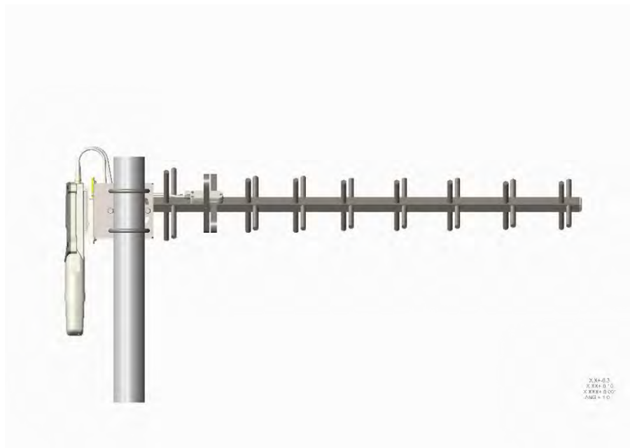
Figure 152: Yagi antenna alignment - upward tilt
