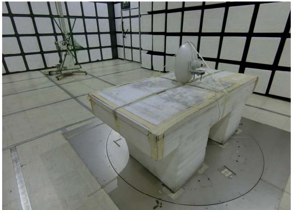
**Test Configuration: Above 1GHz****FRONT VIEW**
