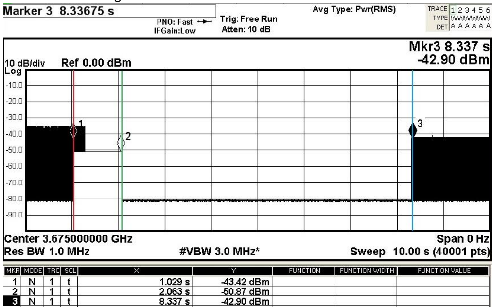
Figure 1-4: TX of at 3675 MHz for 15 MHz channel
