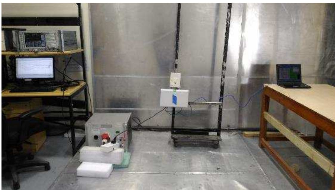
Figure 15: Photograph of Conducted Emission test setup
