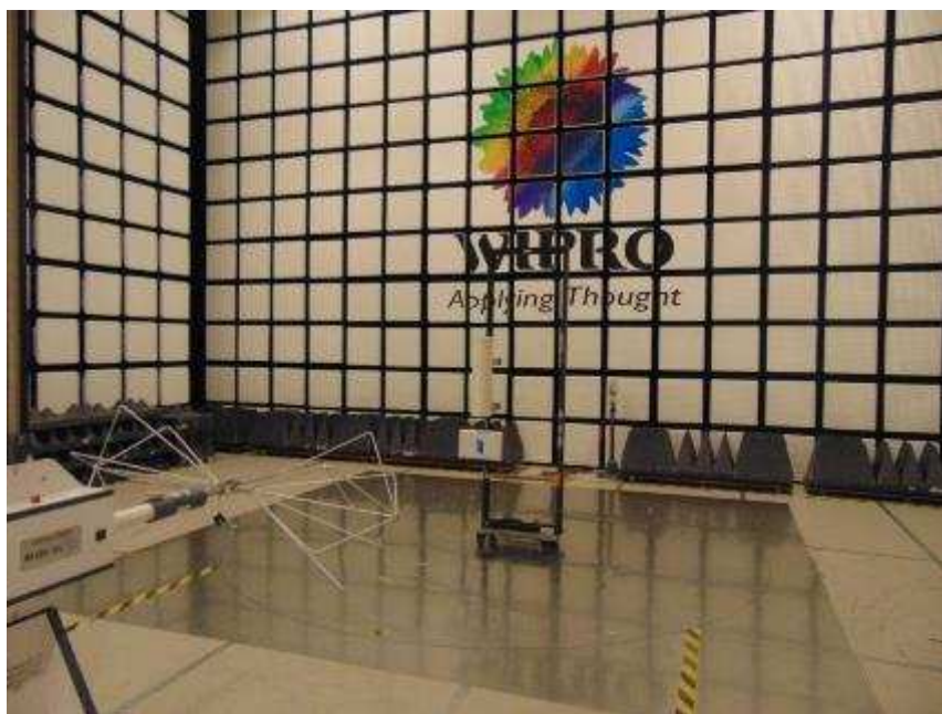
Figure 5: Photograph of Radiated Emission test setup from 30 MHz to 200 MHz - Horizontal polarization
