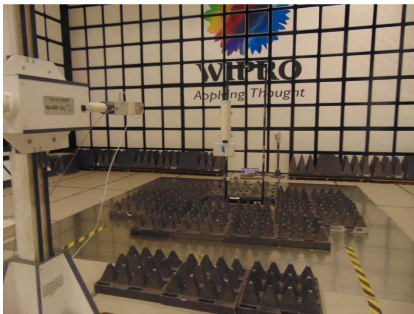
Figure 14: Photograph of Radiated Emission test setup from 26.5 GHz to 40 GHz – Vertical polarization
