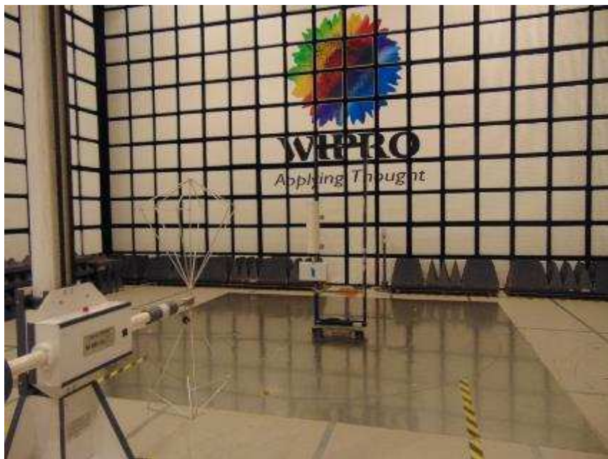
Figure 6: Photograph of Radiated Emission test setup from 30 MHz to 200 MHz - Vertical polarization
