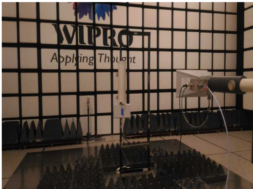
Figure 10: Photograph of Radiated Emission test setup from 1 GHz to 18 GHz -Vertical polarization
