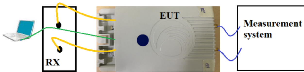
Figure 31: Typical test setup for Conducted RF Test
