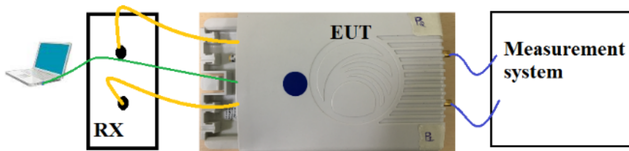
Figure 2: Typical test setup for Conducted RF Test
