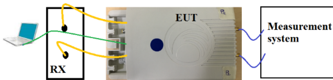
Figure 42: Typical test setup for Conducted Test
