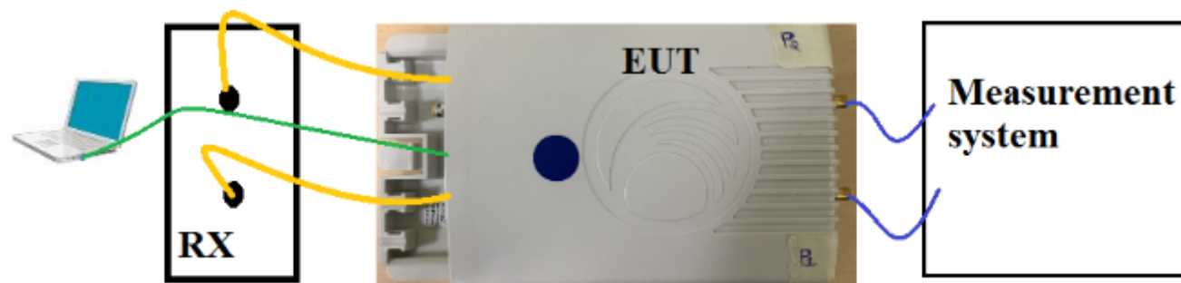
Figure 63: Typical test setup for Conducted test
