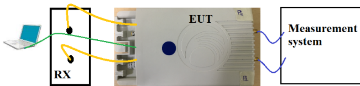
Figure 18 Typical test setup for Conducted RF Test
