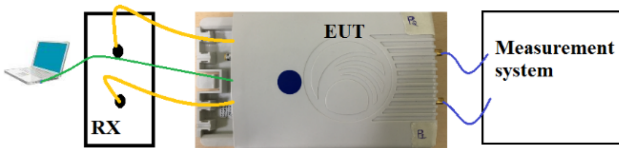
Figure 5: Typical test setup for Conducted RF Test
