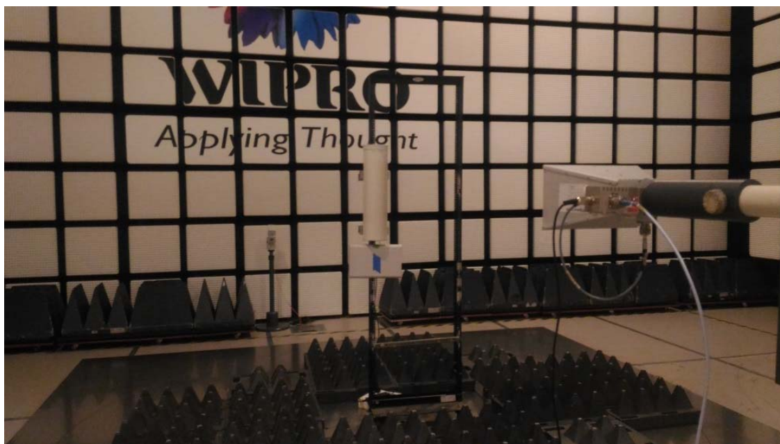
Figure 10: Photograph of Radiated Emission test setup from 1 GHz to 18 GHz -Vertical polarization
