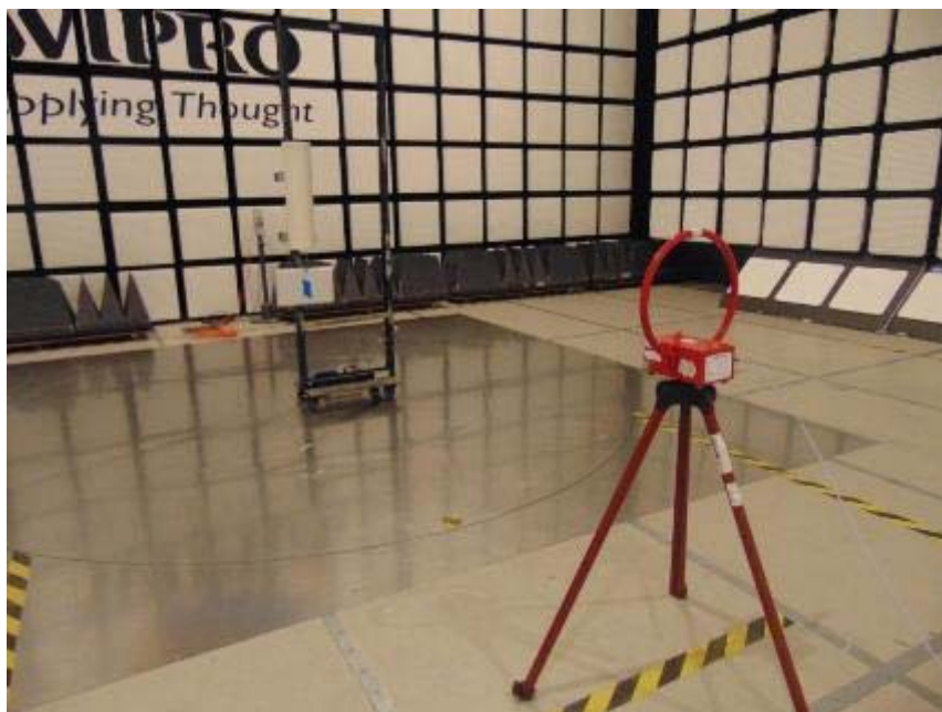
Figure 3: Photograph of Radiated Emission E field measurement test setup from 9 kHz to 30 MHz - parallel
