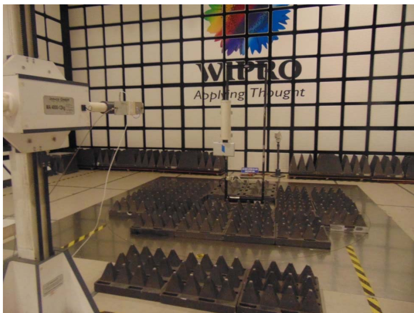
Figure 12: Photograph of Radiated Emission test setup from 18 GHz to 26.5 GHz – Vertical polarization
