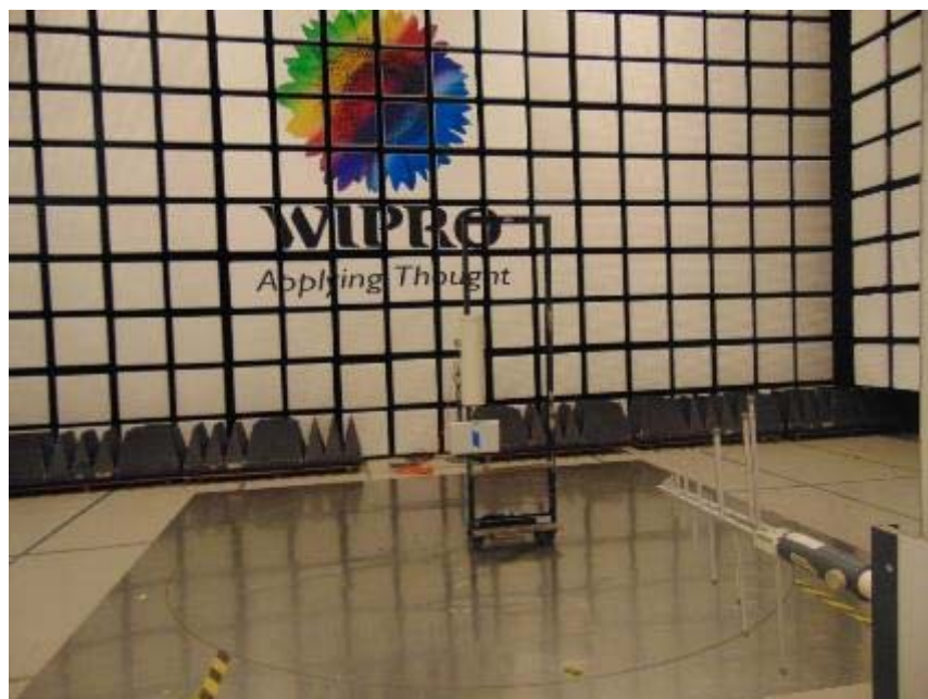
Figure 8: Photograph of Radiated Emission test setup from 200 MHz to 1 GHz -Vertical polarization
