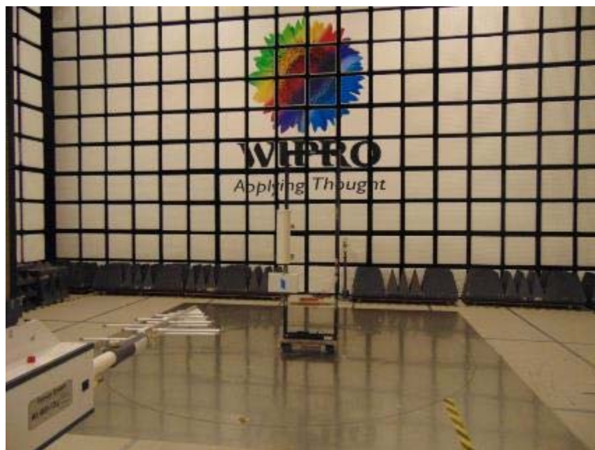
Figure 7: Photograph of Radiated Emission test setup from 200 MHz to 1 GHz -Horizontal polarization
