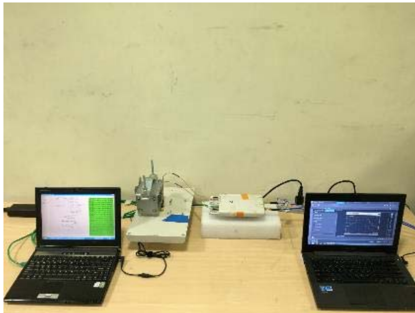
Figure 1: Photograph of conducted measurements test setup-EUT
