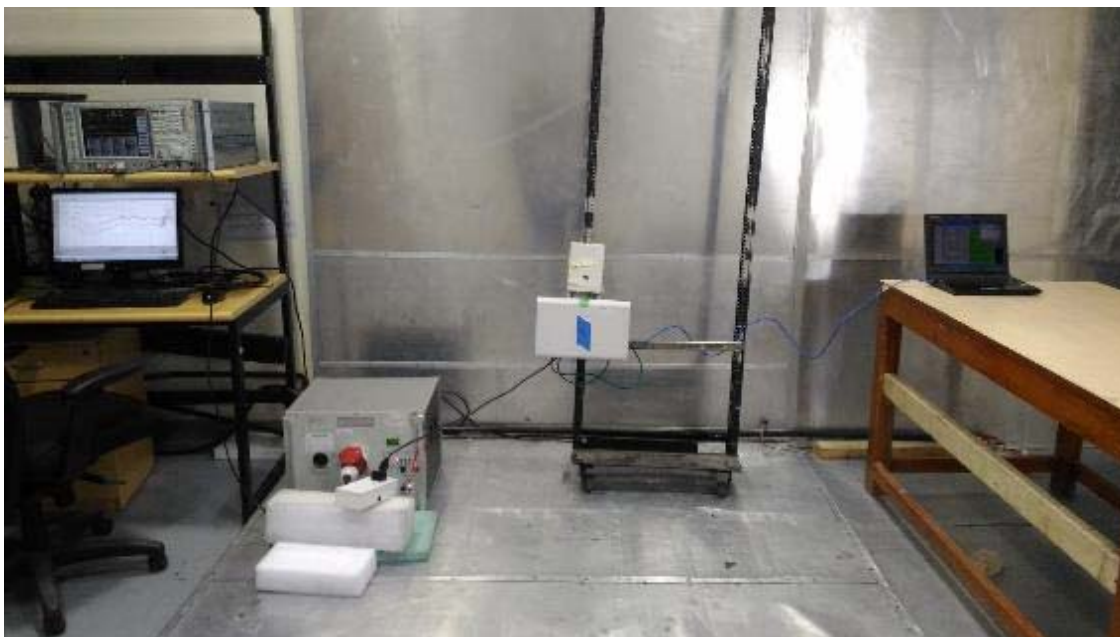
Figure 15: Photograph of Conducted Emission test setup
