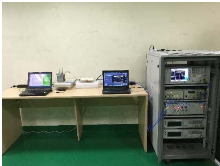
Figure 2: Photograph of conducted measurements test setup-Measurement System
