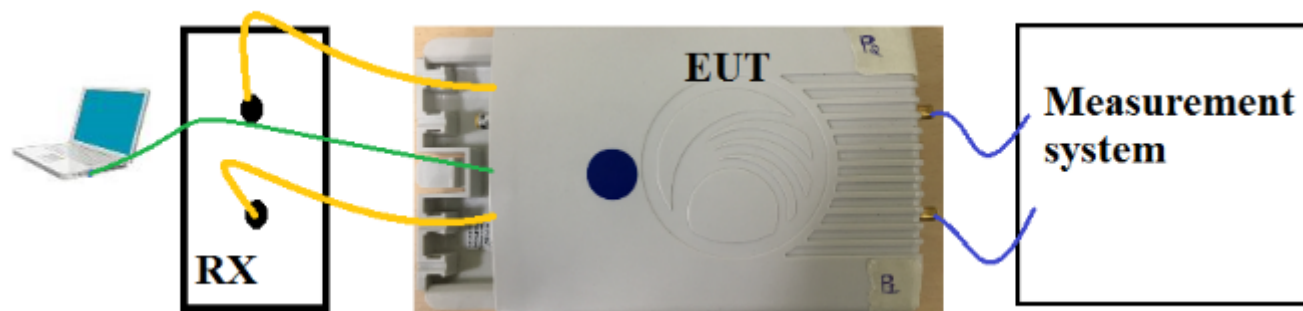
Figure 2: Typical test setup for Conducted RF Test
