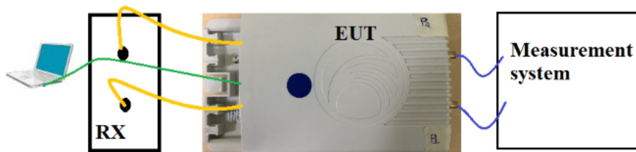
Figure 51: Typical test setup for Conducted Test
