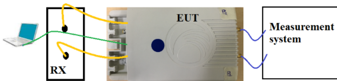
Figure 18 Typical test setup for Conducted RF Test
