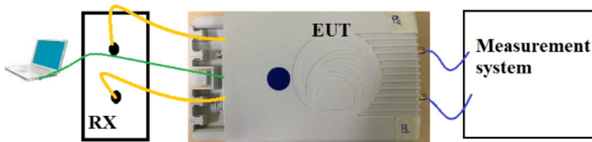
Figure 38: Typical test setup for Conducted Test
