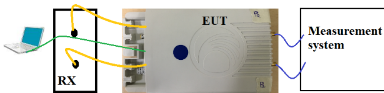
Figure 31: Typical test setup for Conducted RF Test
