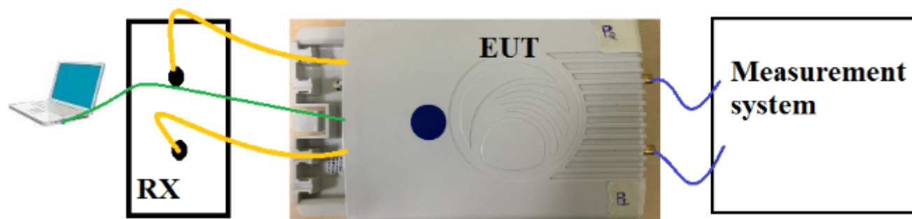
Figure 5: Typical test setup for Conducted RF Test
