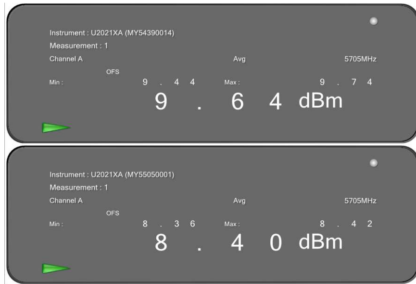
Figure 36: 40 MHz, 17 dBi, High Channel: Maximum conducted output power measured at Ch.0 & Ch.1 – 5705 MHz
