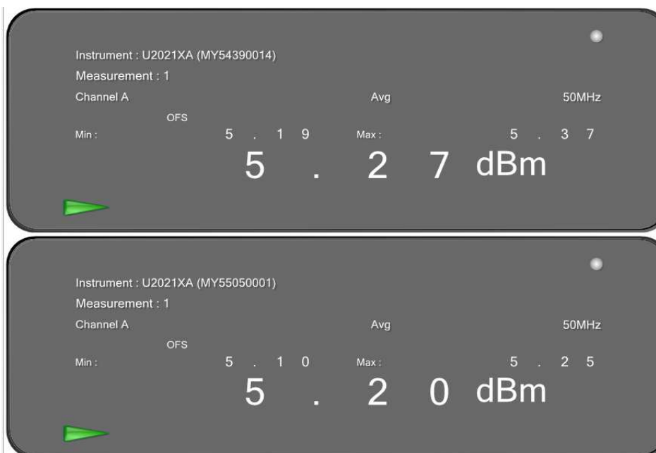
Figure 41: 10 MHz, 17 dBi, High Channel: Maximum conducted output power measured at Ch.0 & Ch.1 – 5720 MHz
