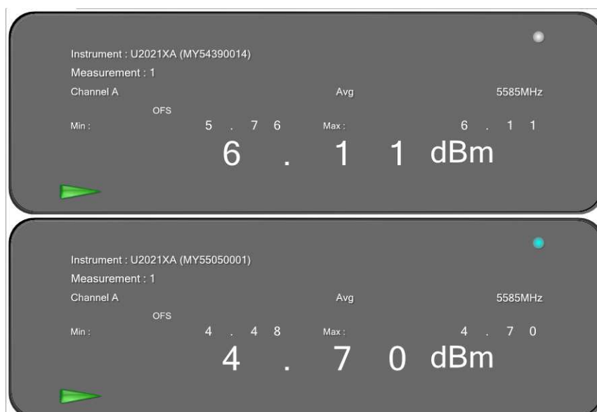
Figure 38: 10 MHz, 17 dBi, Mid Channel: Maximum conducted output power measured at Ch.0 & Ch.1 – 5585 MHz
