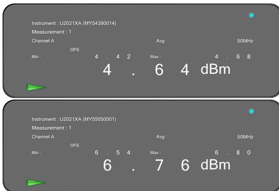
Figure 40: 10 MHz, 17 dBi, Low Channel: Maximum conducted output power measured at Ch.0 & Ch.1 – 5475 MHz
