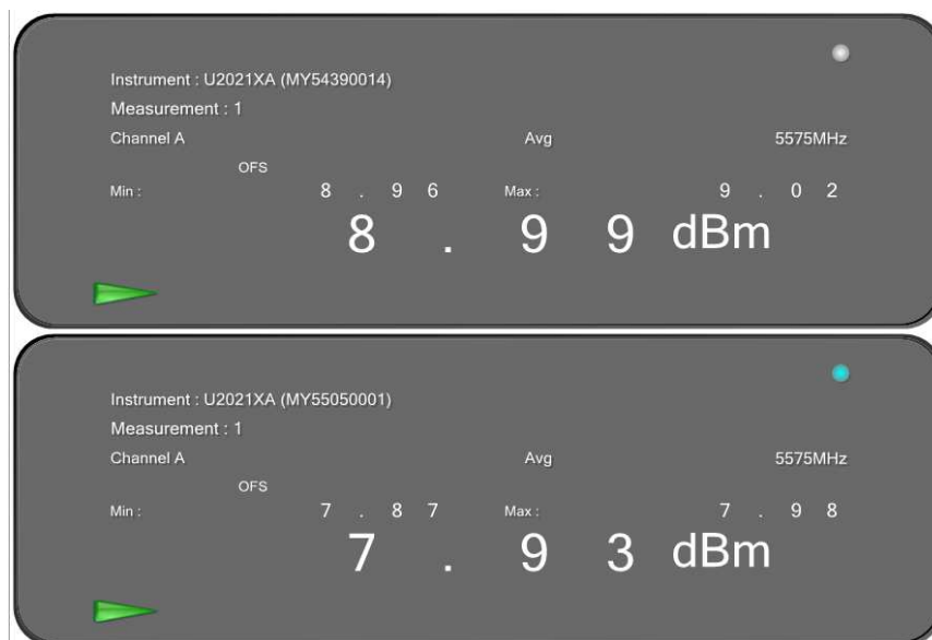
Figure 33: 40 MHz, 17 dBi, Mid Channel: Maximum conducted output power measured at Ch.0 & Ch.1 – 5575 MHz
