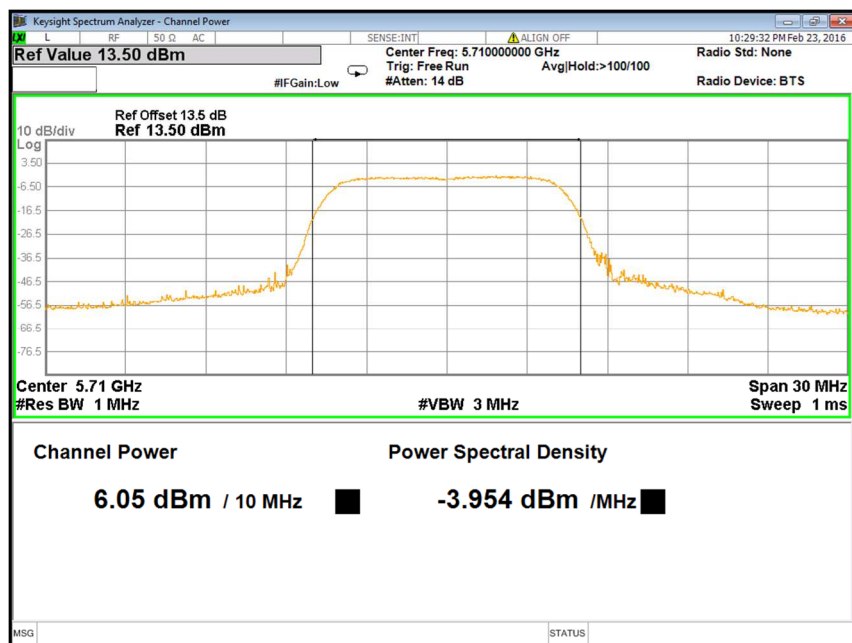
Figure 58: 10 MHz, 17 dBi, High Channel: Power spectral density measured at Ch. 1 – 5710 MHz
