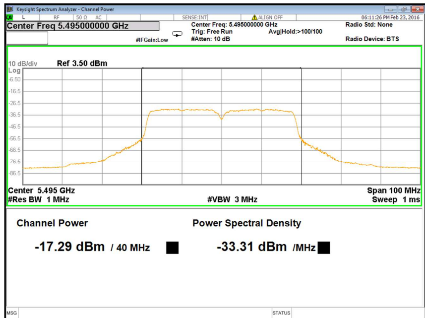
Figure 43: 40 MHz, 17 dBi, Low Channel: Power spectral density measured at Ch. 0 – 5495 MHz
