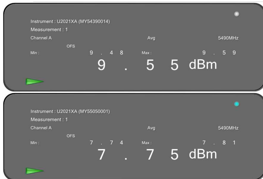
Figure 35: 40 MHz, 17 dBi, Low Channel: Maximum conducted output power measured at Ch.0 & Ch.1 – 5490 MHz
