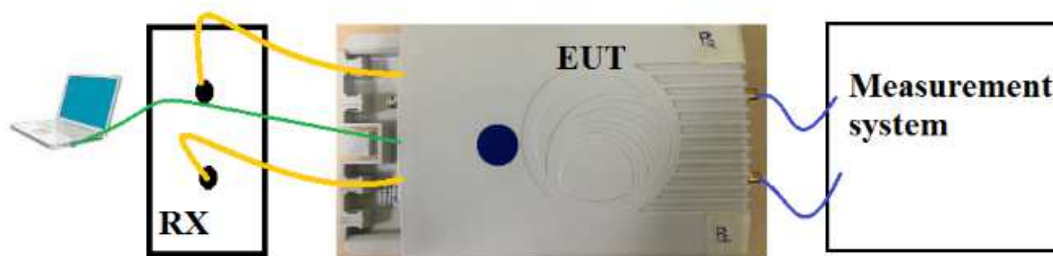
Figure 38: Typical test setup for Conducted Test
