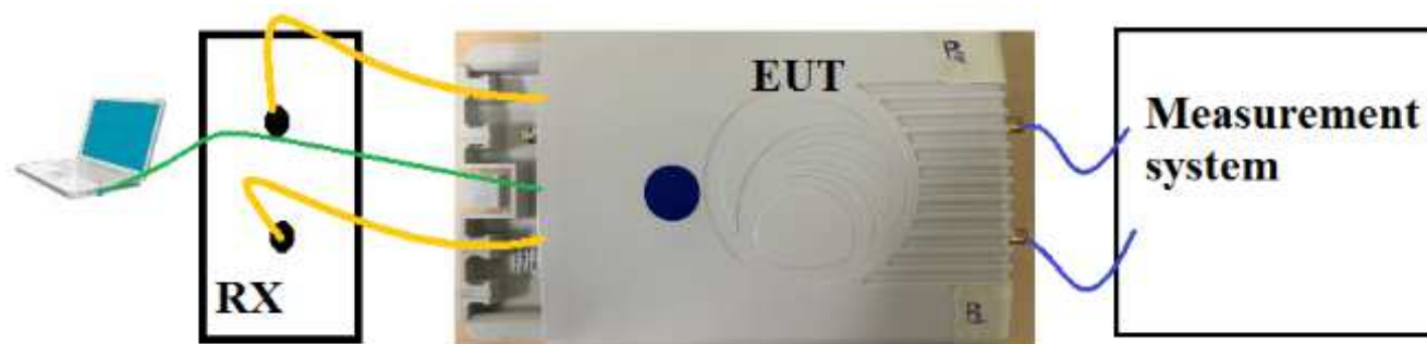
Figure 51: Typical test setup for Conducted Test
