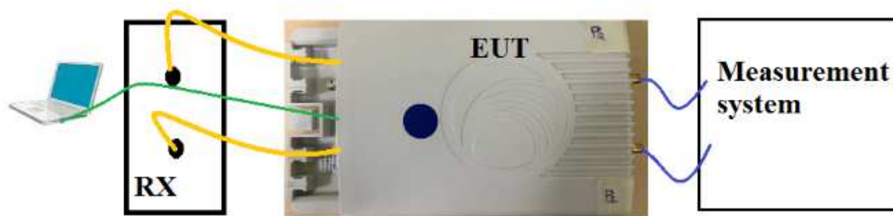
Figure 5: Typical test setup for Conducted RF Test
