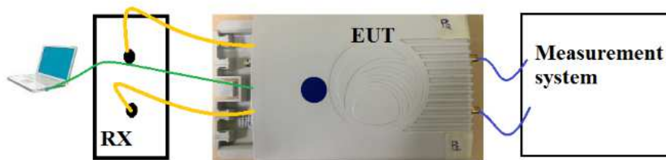
Figure 2: Typical test setup for Conducted RF Test
