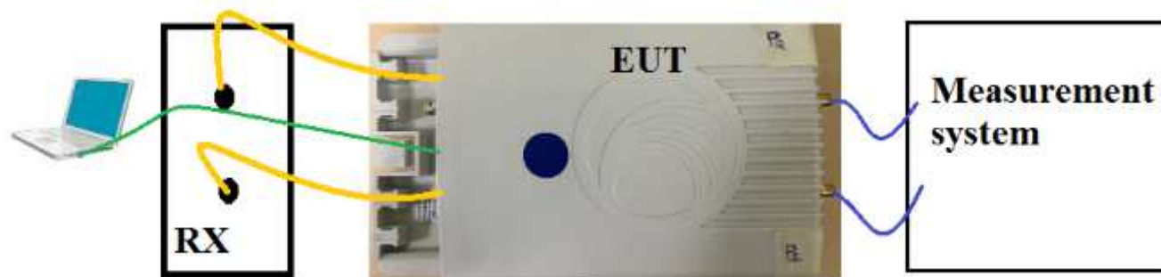
Figure 31: Typical test setup for Conducted RF Test
