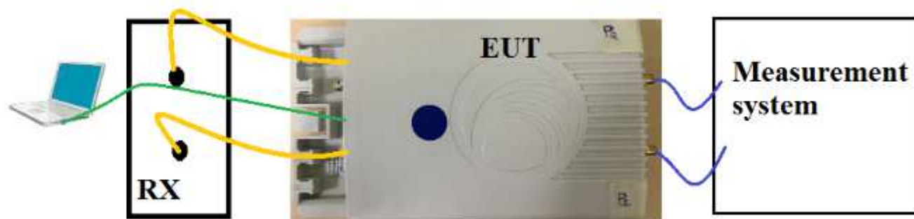
Figure 18 Typical test setup for Conducted RF Test
