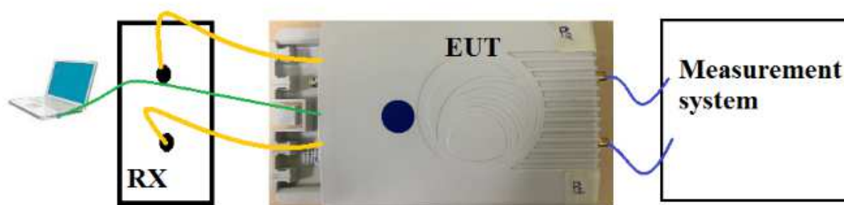
Figure 302: Typical test setup for Conducted Test
