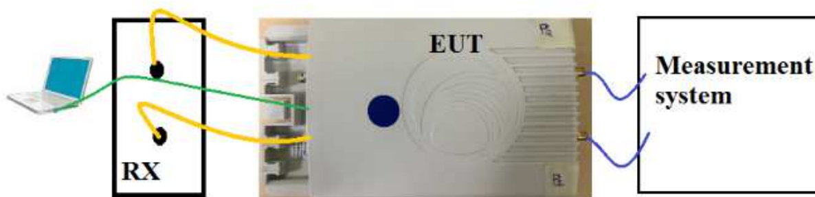
Figure 285: Typical test setup for Conducted Test
