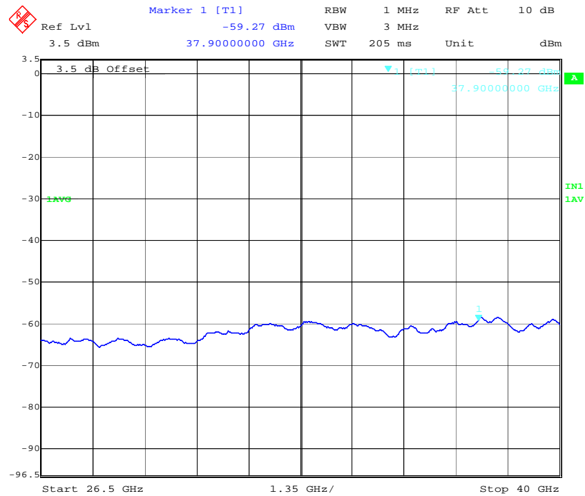
Figure 83: 40MHz, 17dBi, Low Channel: Average Emission from 26.5 GHz to 40 GHz at Ch. 1
