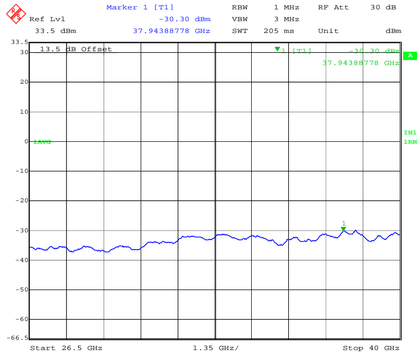
Figure 137: 40MHz, 6dBi, Low Channel: Average Emission from 26.5 GHz to 40 GHz at Ch. 1
