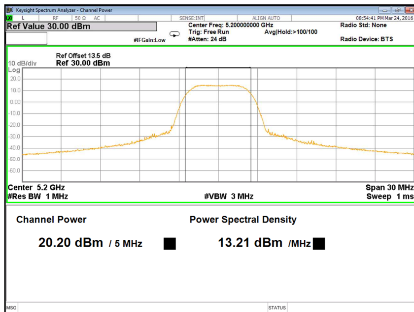
Figure 64: 5MHz, 6dBi, Mid Channel: Power Spectral density Measured at Ch. 0
