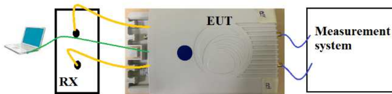
Figure 68: Typical test setup for Conducted Test
