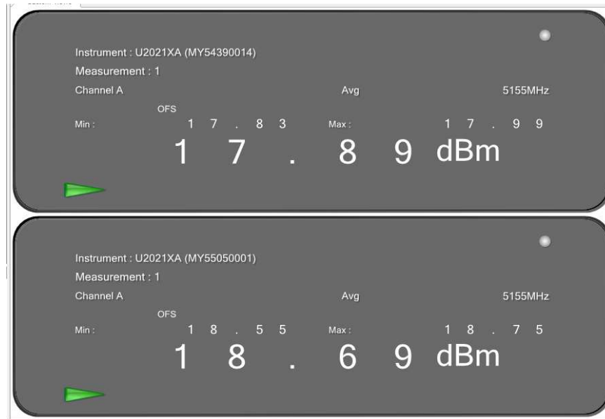
Figure 40: 5MHz, 6dBi, Low Channel: Maximum Conducted Output power Measured at Ch.0 & Ch.1
