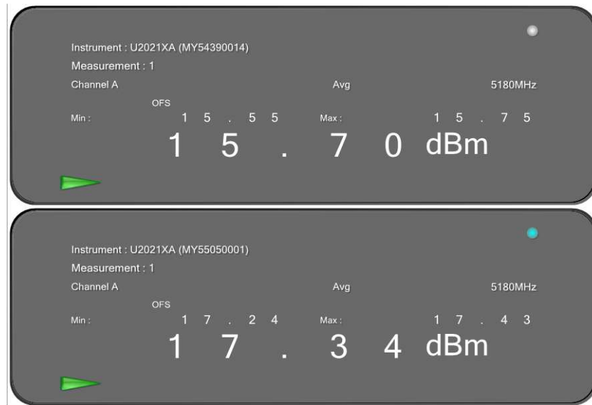
Figure 34: 40MHz, 6dBi, Low Channel: Maximum Conducted Output power Measured at Ch.0 & Ch.1
