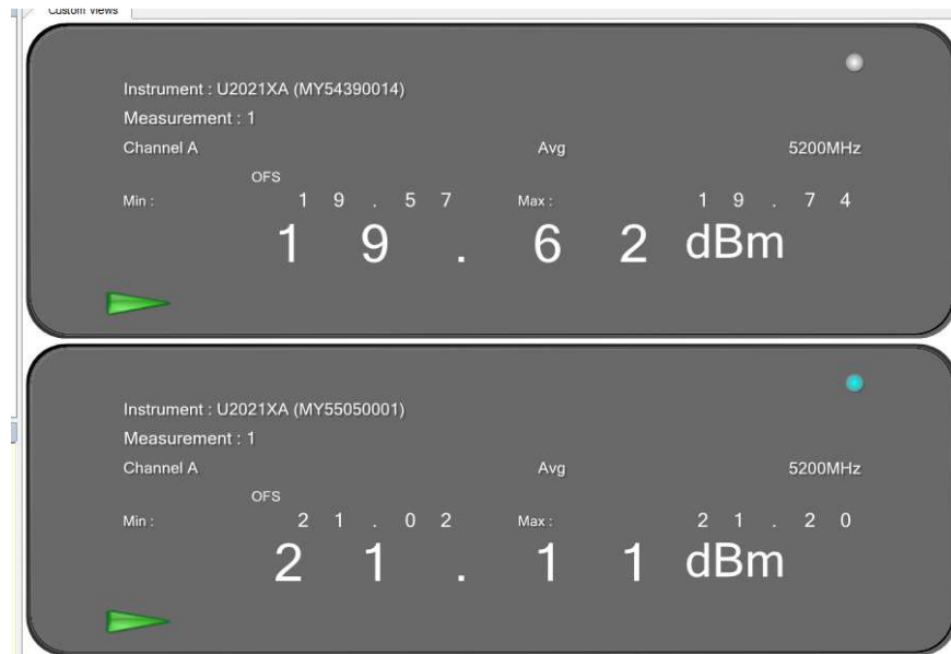
Figure 41: 5MHz, 6dBi, Mid Channel: Maximum Conducted Output power Measured at Ch.0 & Ch.1
