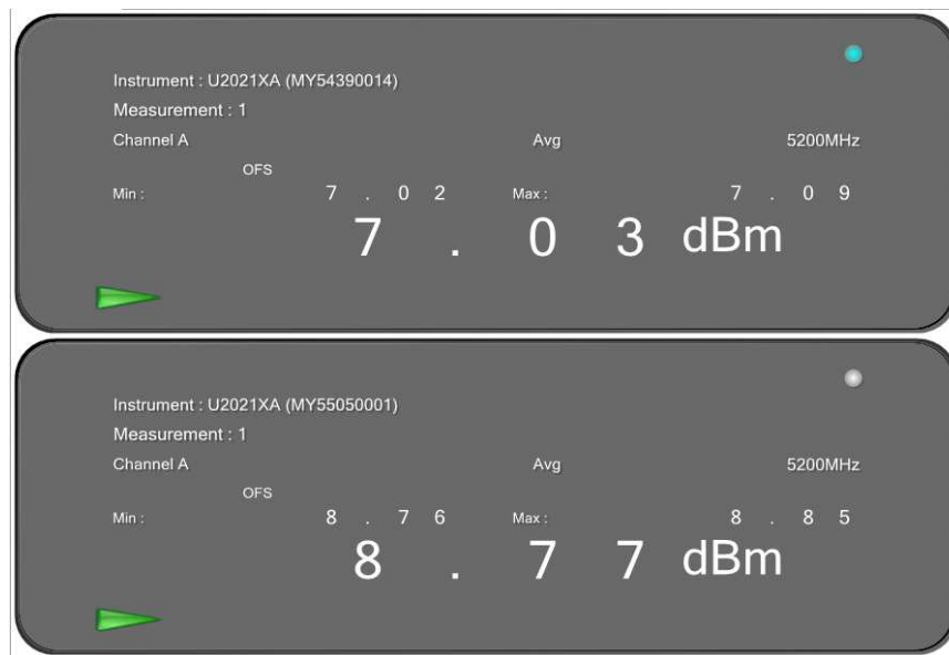
Figure 33: 40MHz, 17dBi, High Channel: Maximum Conducted Output power Measured at Ch.0 & Ch.1
