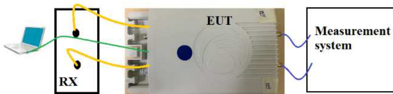
Figure 2: Typical test setup for Conducted RF Test
