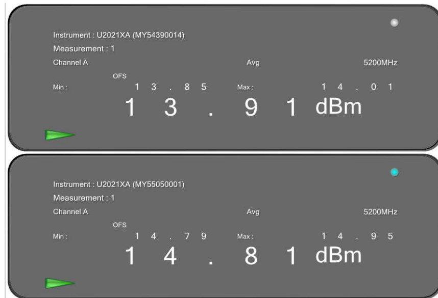
Figure 35: 40MHz, 6dBi, Mid Channel: Maximum Conducted Output power Measured at Ch.0 & Ch.1
