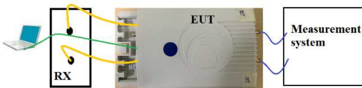
Figure 43: Typical test setup for Conducted Test
