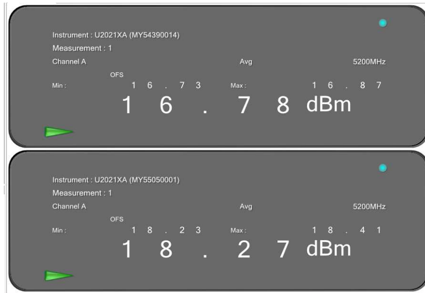
Figure 36: 40MHz, 6dBi, High Channel: Maximum Conducted Output power Measured at Ch.0 & Ch.1
