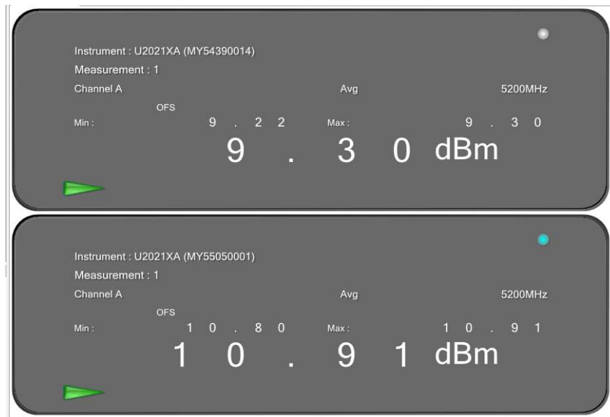
Figure 38: 5MHz, 17dBi, Mid Channel: Maximum Conducted Output power Measured at Ch.0 & Ch.1
