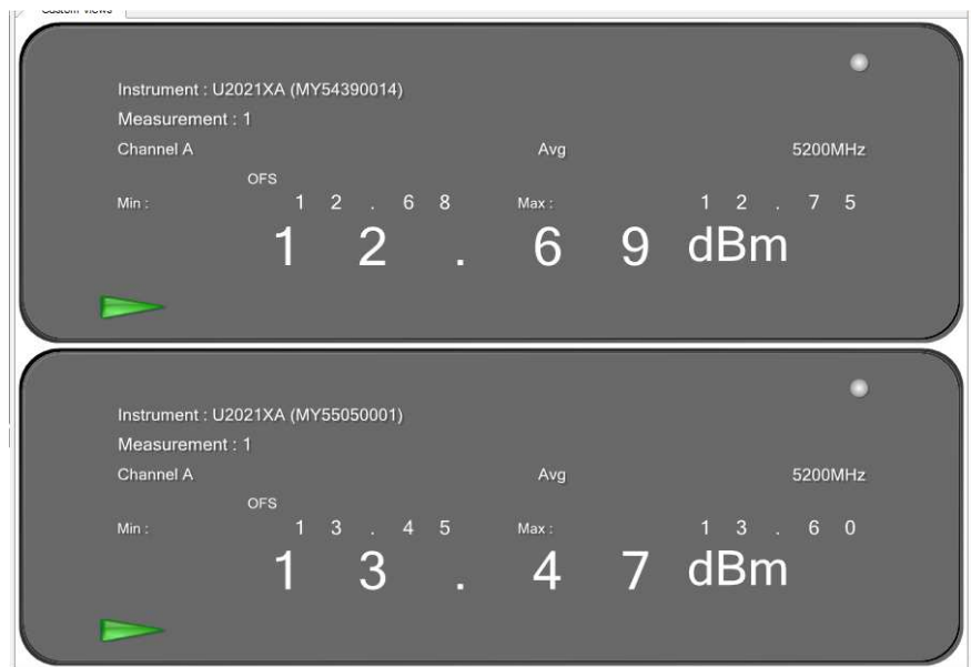
Figure 32: 40MHz, 17dBi, Mid Channel: Maximum Conducted Output power Measured at Ch.0 & Ch.1
