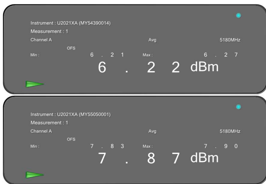
Figure 31: 40MHz, 17dBi, Low Channel: Maximum Conducted Output power Measured at Ch.0 & Ch.1
