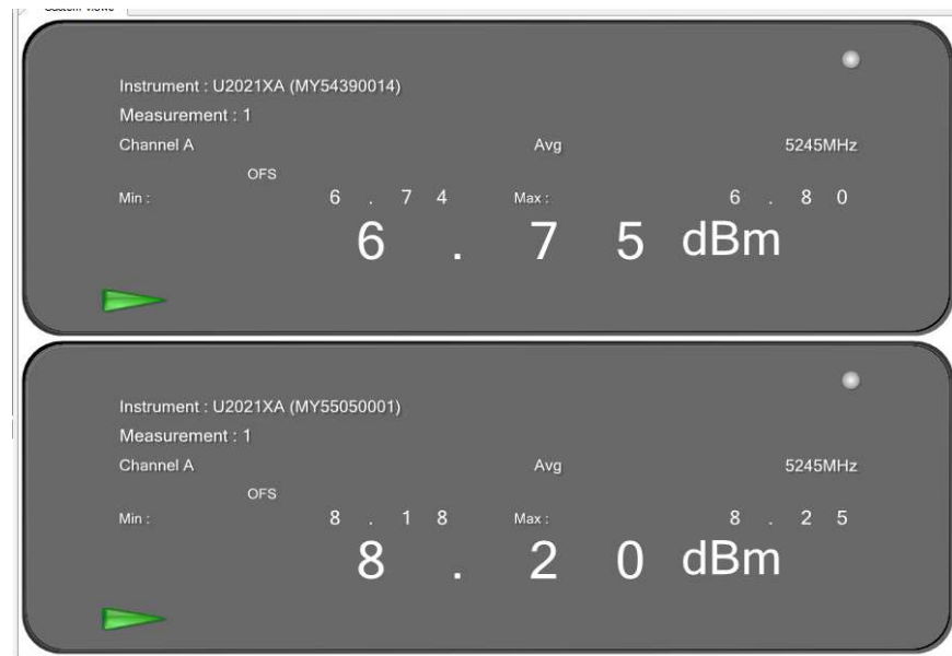
Figure 39: 5MHz, 17dBi, High Channel: Maximum Conducted Output power Measured at Ch.0 & Ch.1
