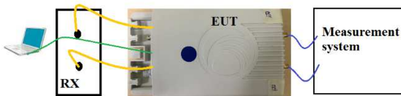
Figure 30: Typical test setup for Conducted RF Test
