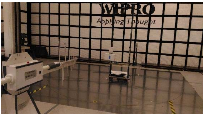
Figure 8 Test setup for Radiated Emission test from 200MHz to 1GHz -Vertical Polarization
