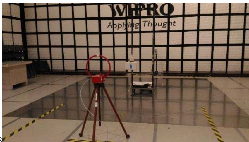
Figure 3 Test setup for Radiated Emission E field measurement from 9 kHz to 30MHz – Parallel
