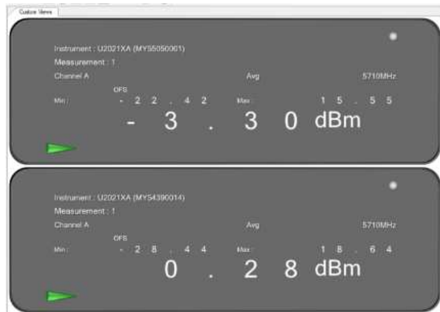
Figure 94: Maximum Conducted Output power measured at ch.0 & ch.1
