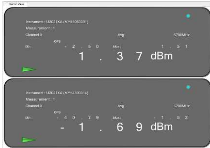
Figure 79: Maximum Conducted Output power measured at ch.0 & ch.1
