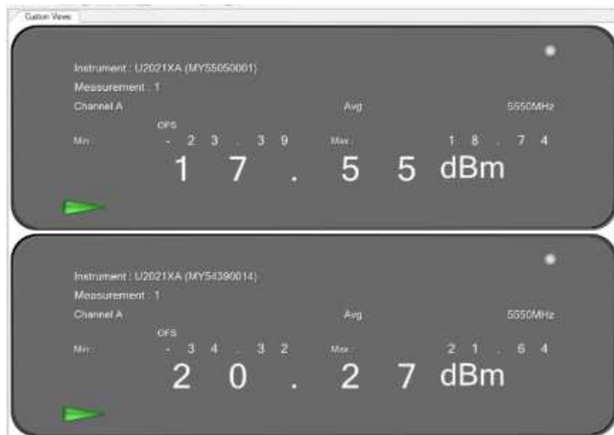
Figure 78: Maximum Conducted Output power measured at ch.0 & ch.1
