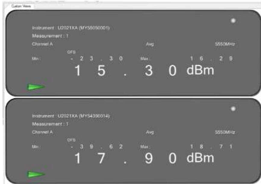
Figure 81: Maximum Conducted Output power measured at ch.0 & ch.1
