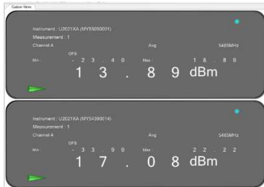
Figure 80: Maximum Conducted Output power measured at ch.0 & ch.1
