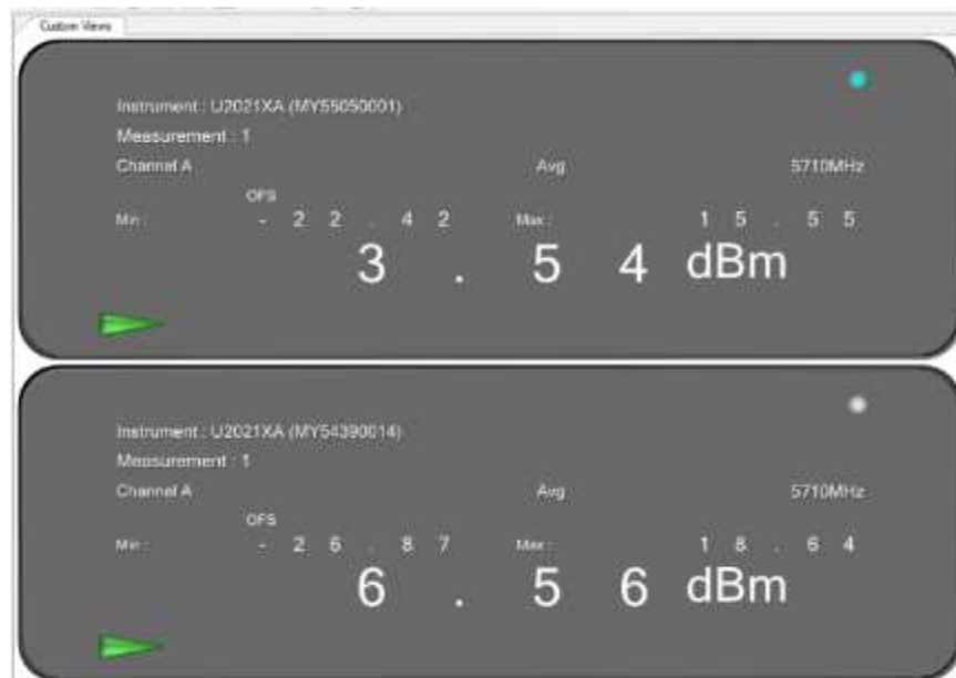
Figure 88: Maximum Conducted Output power measured at ch.0 & ch.1
