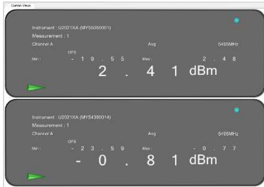
Figure 77: Maximum Conducted Output power measured at ch.0 & ch.1
