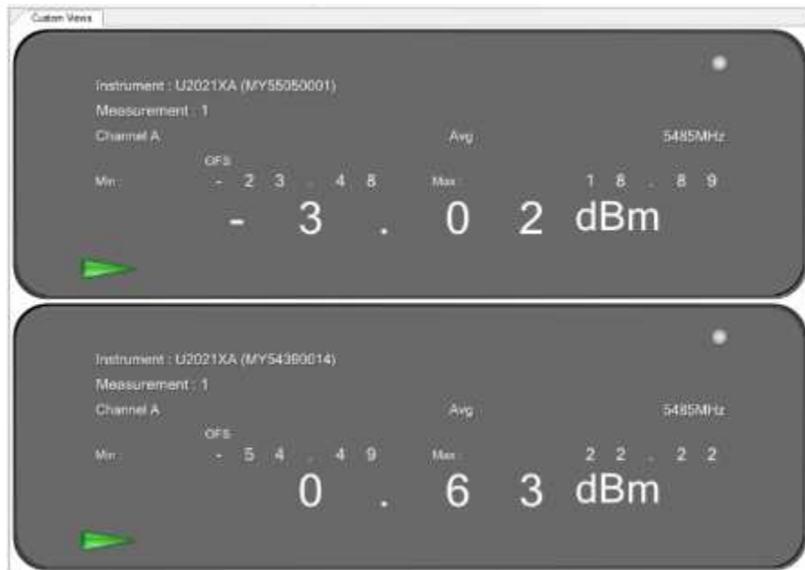
Figure 92: Maximum Conducted Output power measured at ch.0 & ch.1
