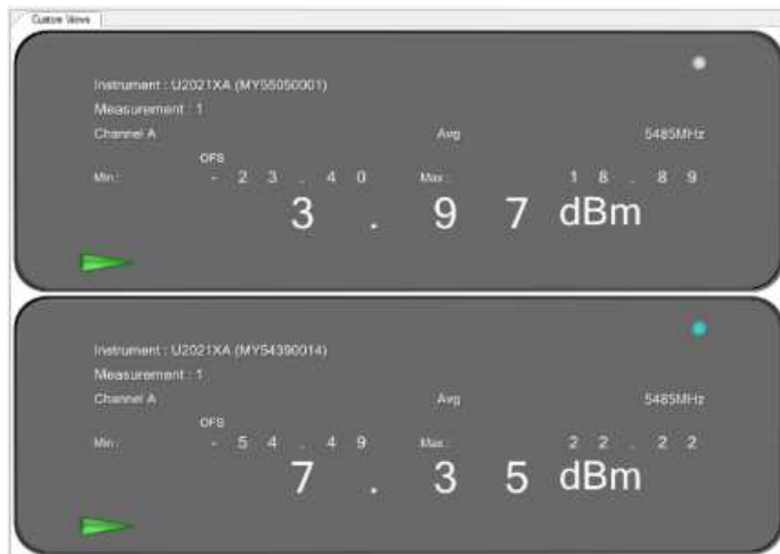
Figure 86: Maximum Conducted Output power measured at ch.0 & ch.1
