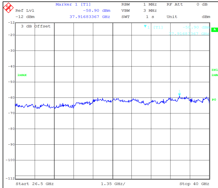
Figure 47: Emission measured with Peak Detector from 26.5GHz to 40GHz at Ch. 0
