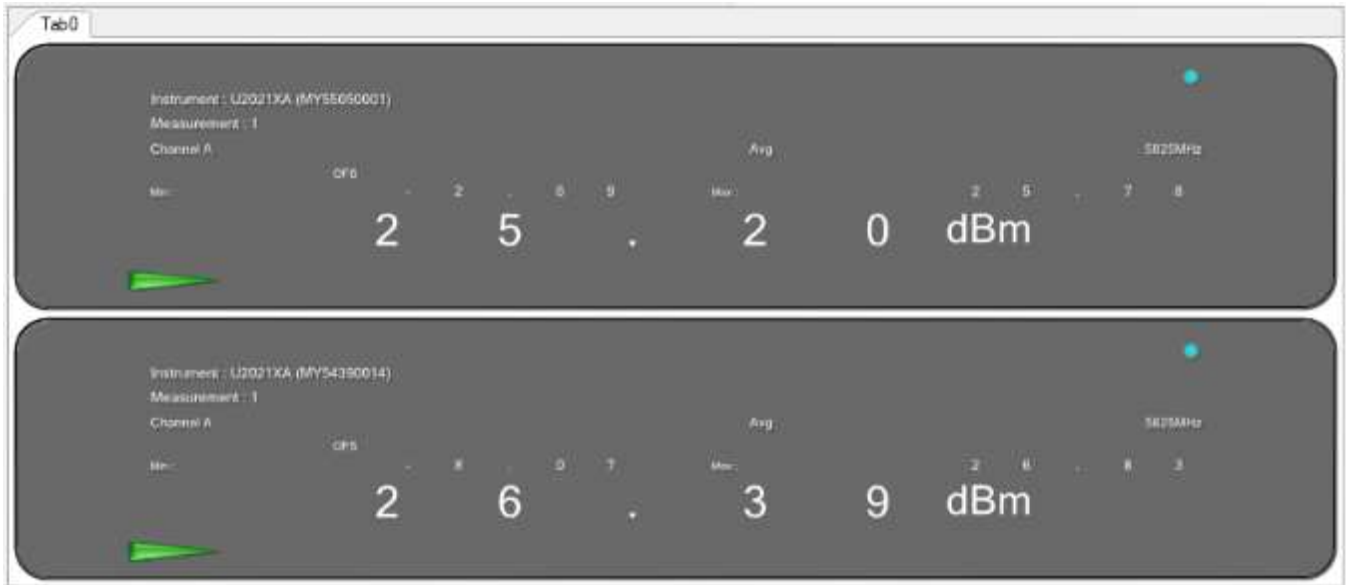
Figure 343: Maximum Conducted Output power measured at Ch.0 & Ch.1
