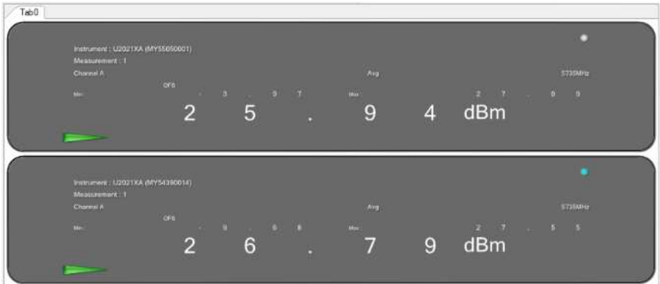
Figure 344: Maximum Conducted Output power measured at Ch.0 & Ch.1
