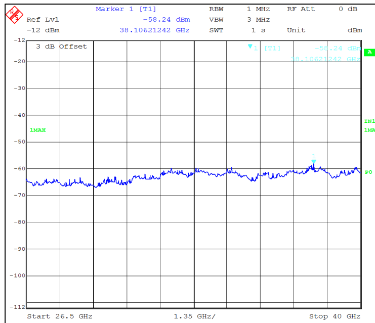
Figure 272: Emission measured with Peak Detector from 26.5GHz to 40GHz at Ch. 1
