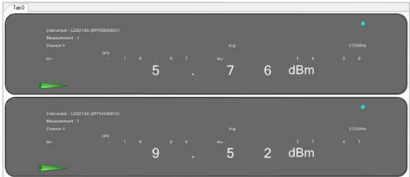
Figure 356: Maximum BW Conducted Output power measured at Ch.0 & Ch.1
