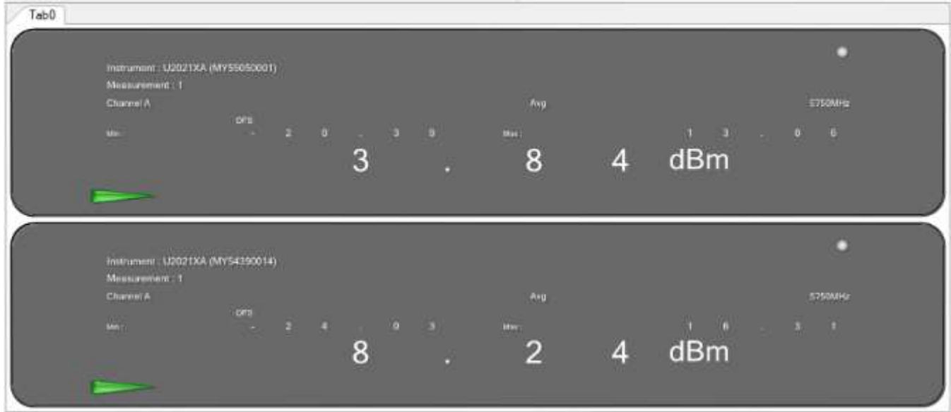
Figure 353: Maximum Conducted Output power measured at Ch.0 & Ch.1
