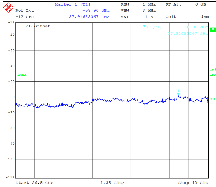
Figure 263: Emission measured with Peak Detector from 26.5GHz to 40GHz at Ch. 0
