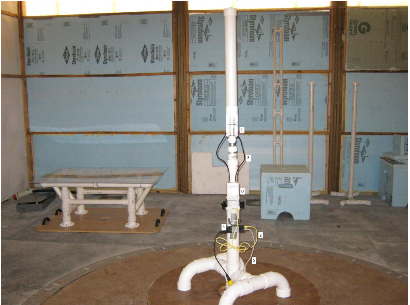
Radiated with Omni Antenna - Back, below 1 GHz
